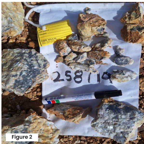
Figure 2: Sample 258119 – Calcite-quartz mineralisation with assays returning 17% Sb & Figure 3: Stibnite Mullock near adit entrance
