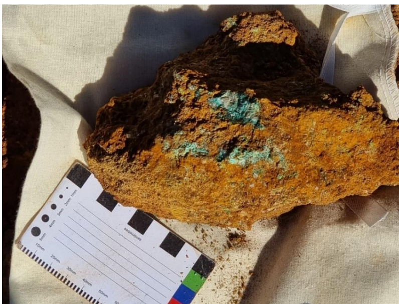
Figure 4: Rock Chip sample WM24-22 which returned 23.8% copper and 4.00g/t gold.
