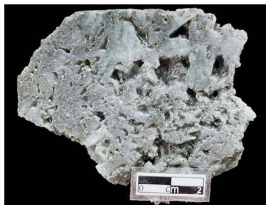
ARD009 (80.1m); core specimen of bladed vuggy, quartz vein. From within a 0.6m interval that assayed 14.95 g/t Au and 15.5 g/t Ag (79.9-80.5m)
