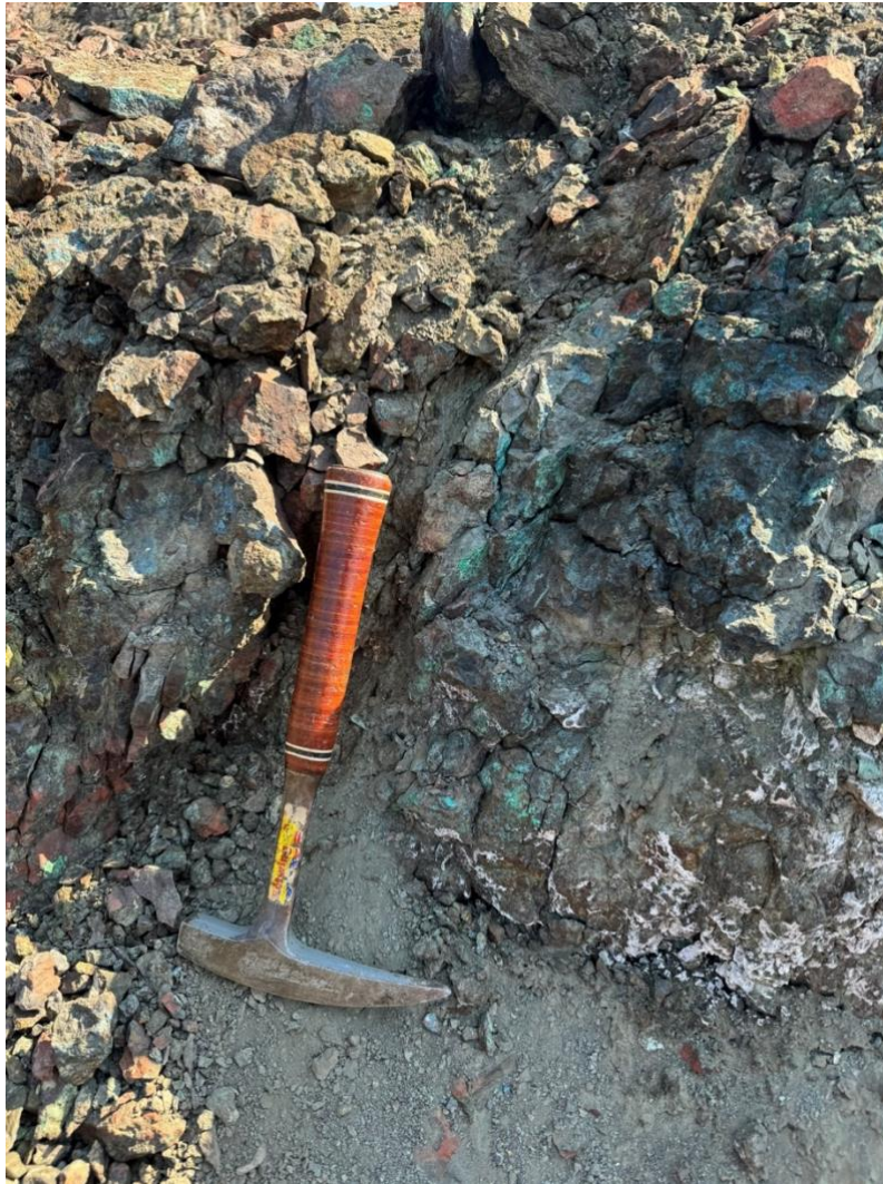
Figure 10: Outcrop photograph for sample F005408 illustrating a brick red K-feldspar-skarn breccia with abundant copper secondary minerals after chalcopyrite-bornite-chalcocite sulphides. Sample returned 233g/t Ag, 9.82% Cu, 1.67% Pb, 2.35% Zn .
