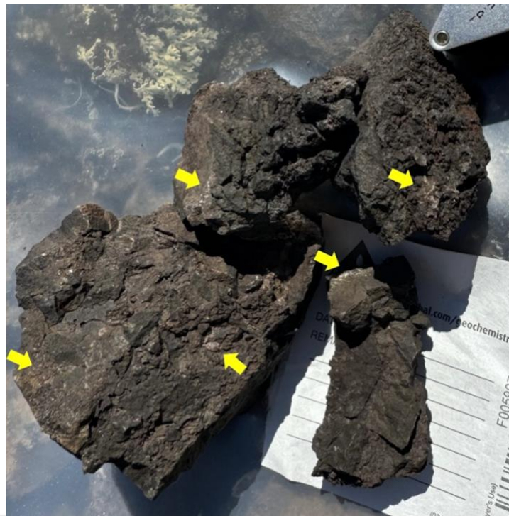
Figure 9: Photograph of sample F005907 which returned 7.54% Ag from the Spud Silver occurrence. Silver present within the chlorite altered host rock and within the breccia cement phase alongside calcite. Yellow arrows point to visible native silver.
