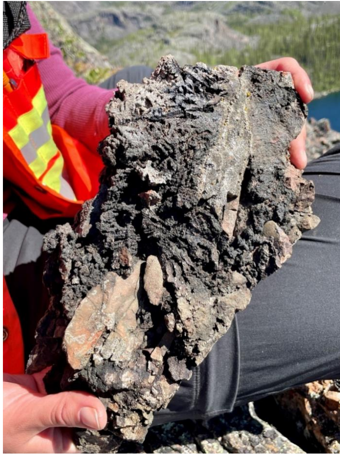
Figure 8: Photograph of sample F005909 which returned 5.35% Ag. Tarnished native silver and calcite cement can be observed between the clasts of potassic altered diorite.
