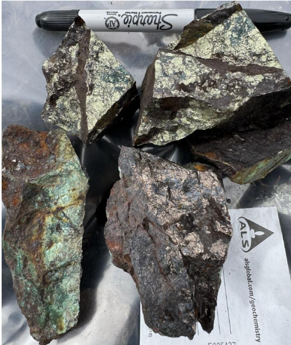
Figure 6: Photograph of sample F005437 with massive bornite-chalcopyrite which returned 42.60% Cu, 2.28g/t Au, 159g/t Ag, 0.364% Co from the Glacier IOCG trend.
