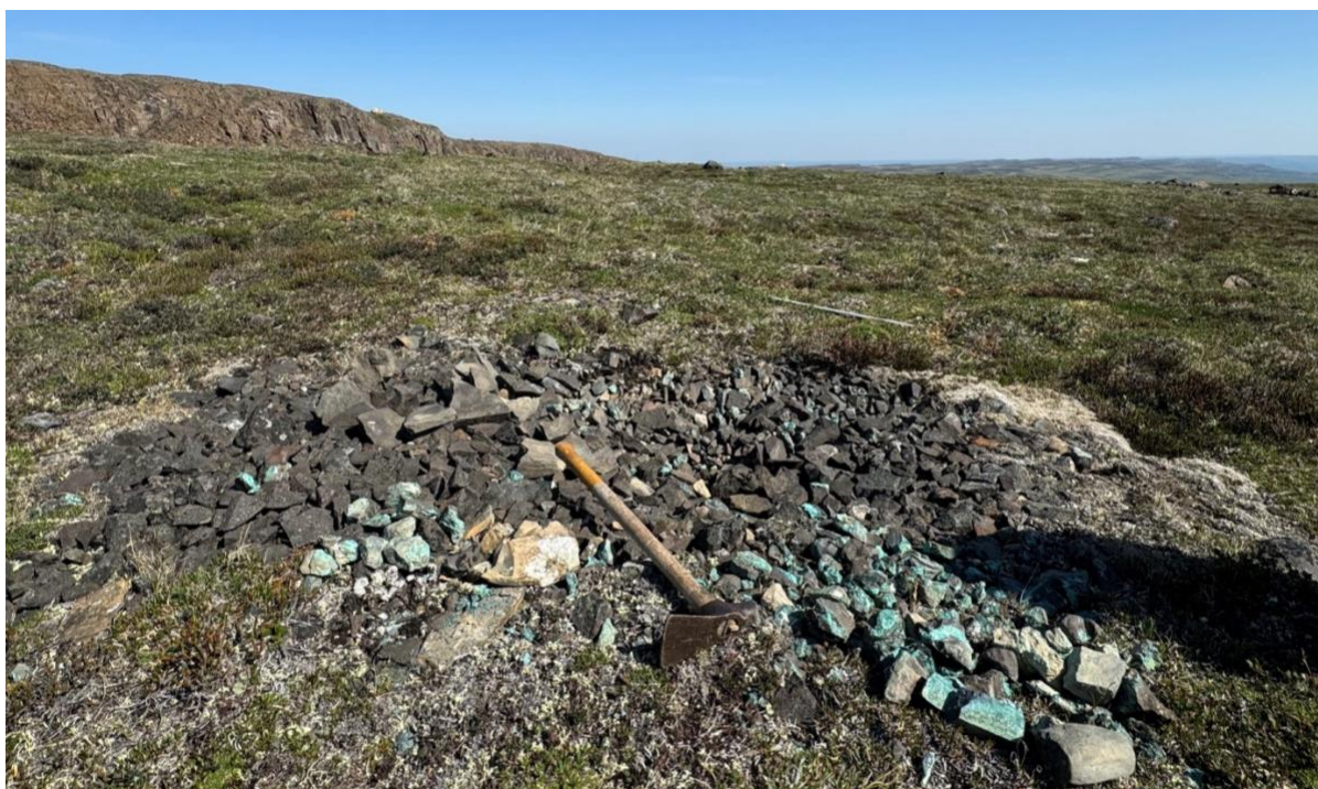
Figure 3: Photograph of frost heaved mineralisation at the site of sample F005921. Semi-massive chalcocite veining returned 54.02% Cu and 34g/t Ag
