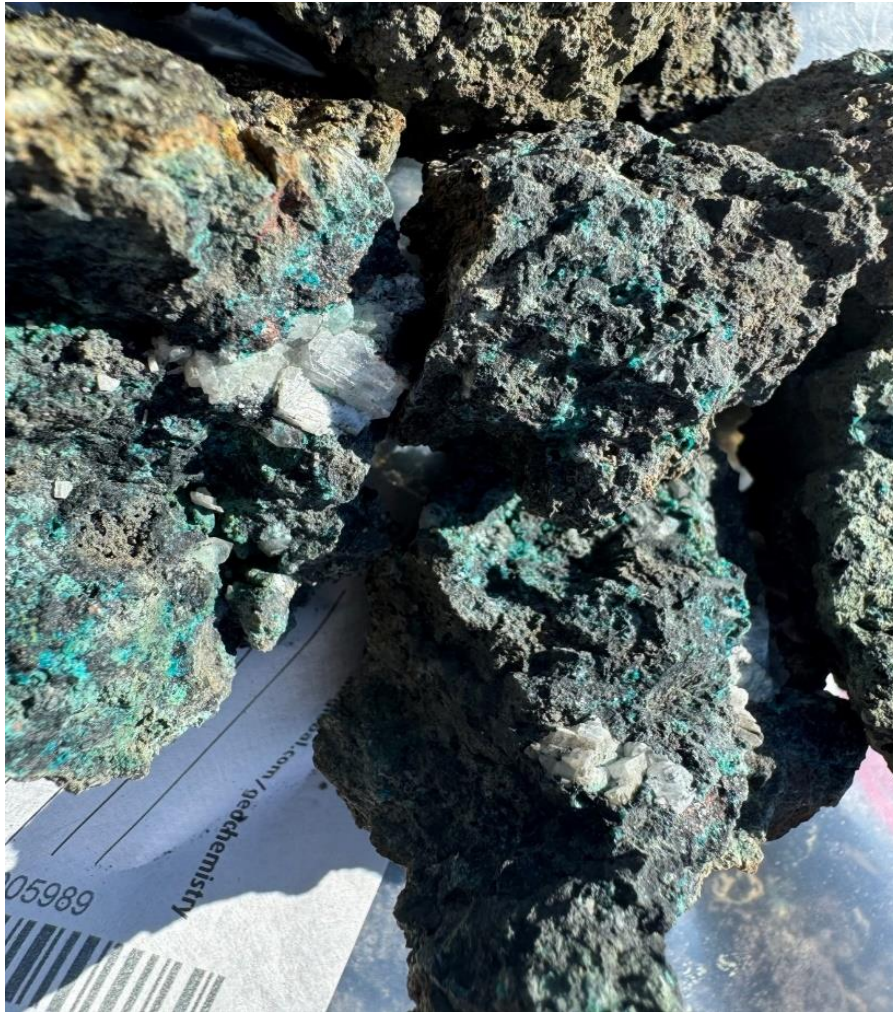
Figure 2: Photograph of sample F005989, taken from a basalt flow top with replacement style copper mineralisation at the Wanda District. The sample includes native copper, returning 9.63% Cu
