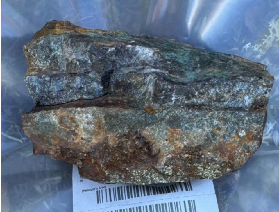
Figure 7: Photograph of sample F005669, quartz-sulphide veining from Coyote which returned 16.95g/t Au, 45.3g/t Ag and 10.55% Cu.
