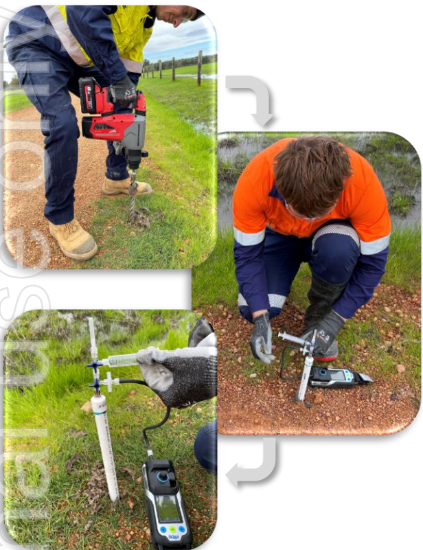
Spot soil gas sampling equipment
