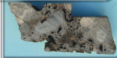
Mudstone core of the Bundella Correlate section @957.5m displaying vuggy porosity
