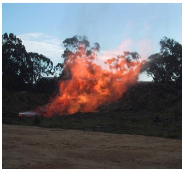
Figure 2: Flaring of gas at the Wombat-1 Gas Well
