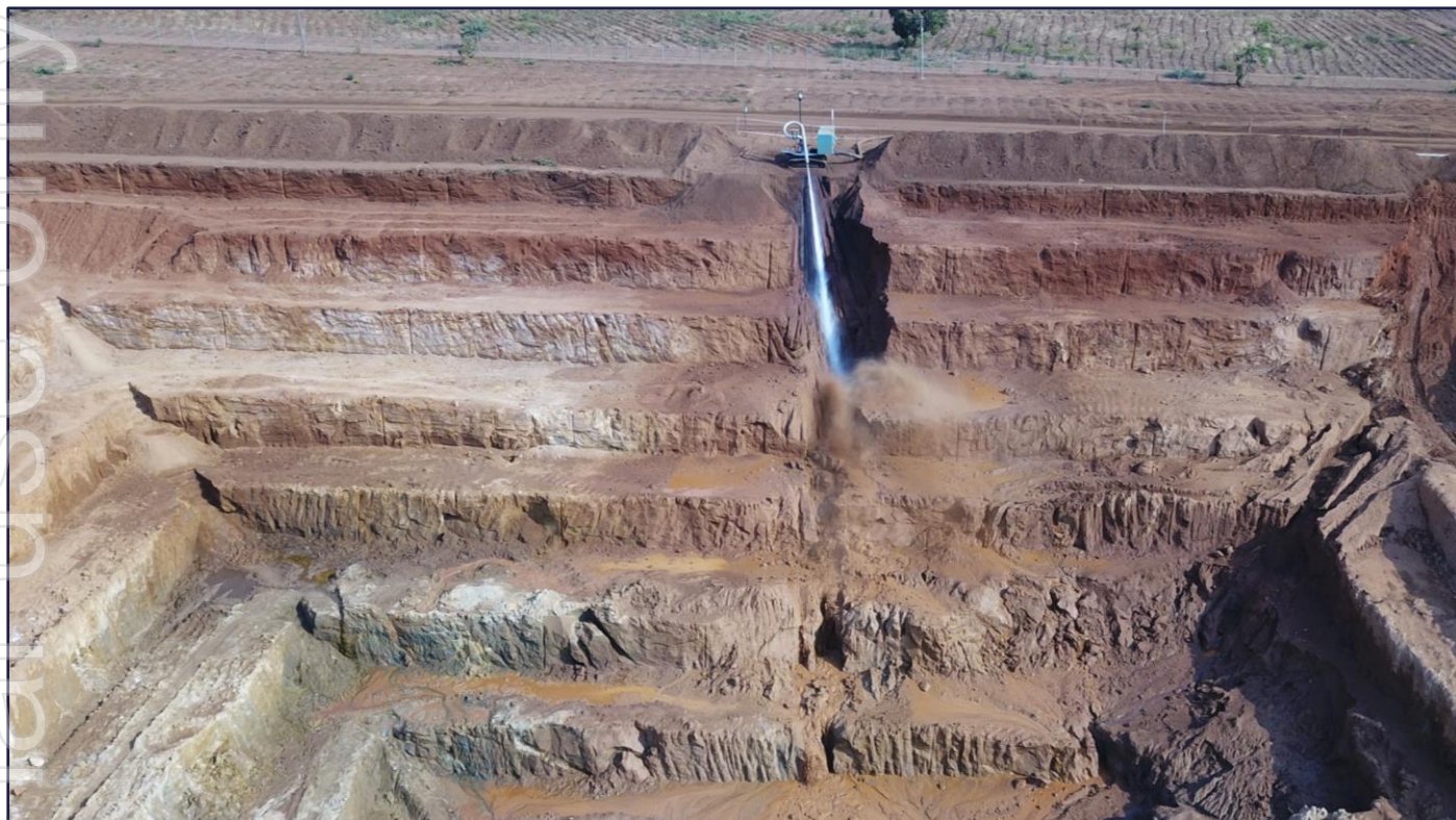
Figure 5: Hydraulic mined material (slurry) flowing freely to the collection point in the bottom of the sump
