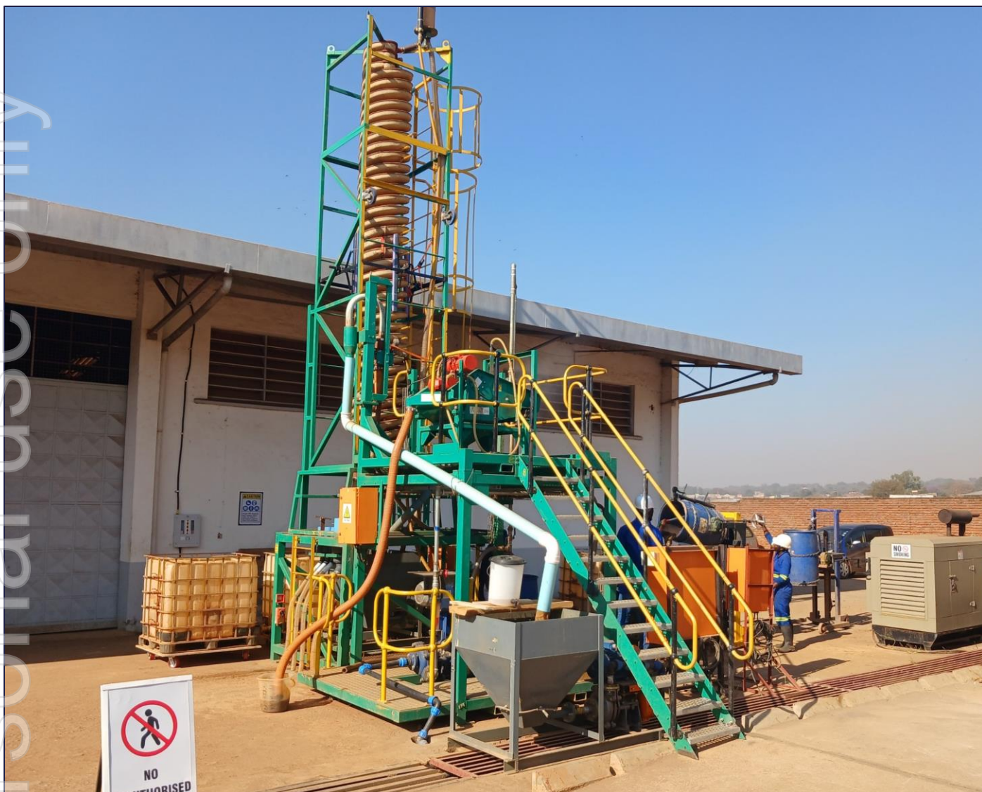
Figure 2: Spiral Plant installed at Sovereign's Lilongwe facility
