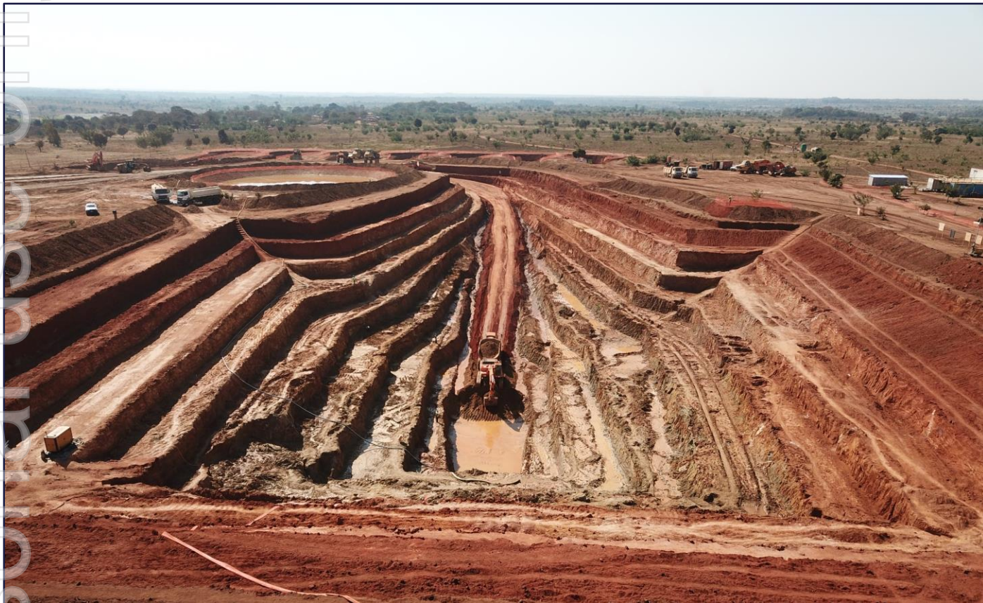
Figure 3: Kasiya Pilot Phase Test Pit mined to 20 metres depth
