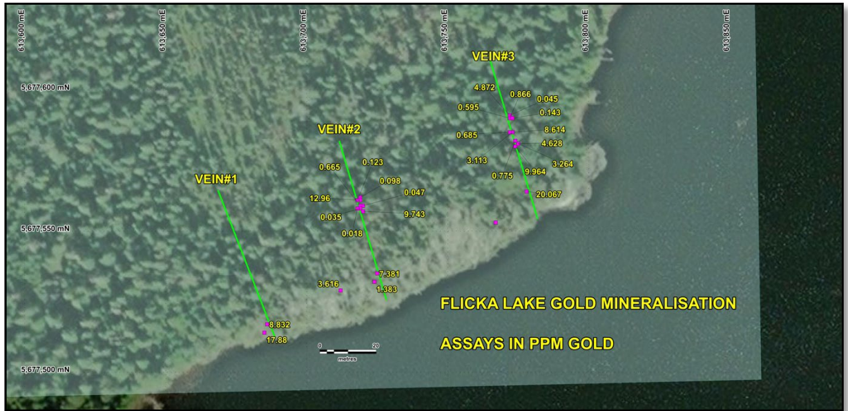
Figure 1: Flicka Lake Claim area with historical channel and grab samples results in ppm Au (equivalent to g/t Au)
