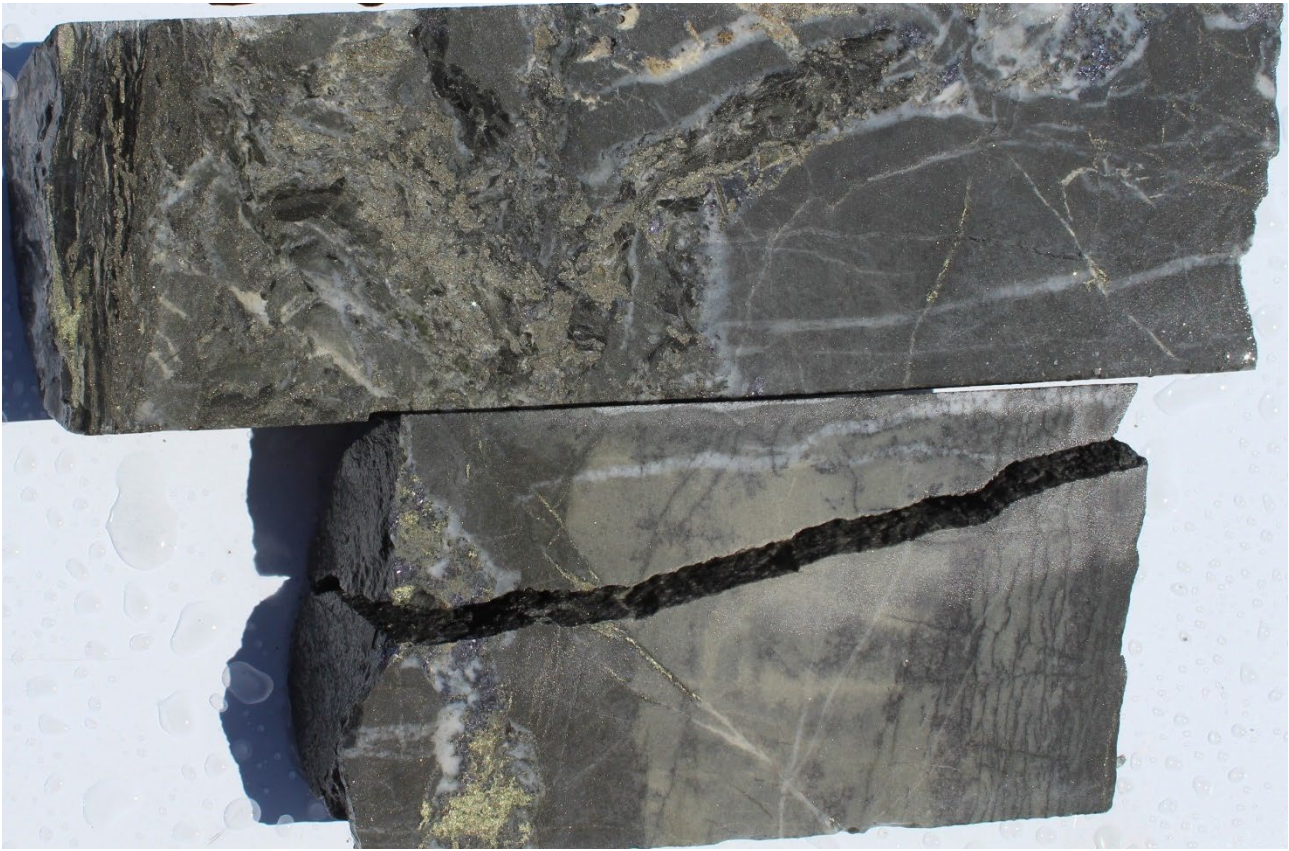
Figure 11: WDR CDD001 from 203.3-203.6m, with pyrite-galena-sphalerite and chalcopyrite with sericite-silica alteration. Possible later, cross-cutting chalcopyrite dominant veins were observed.
