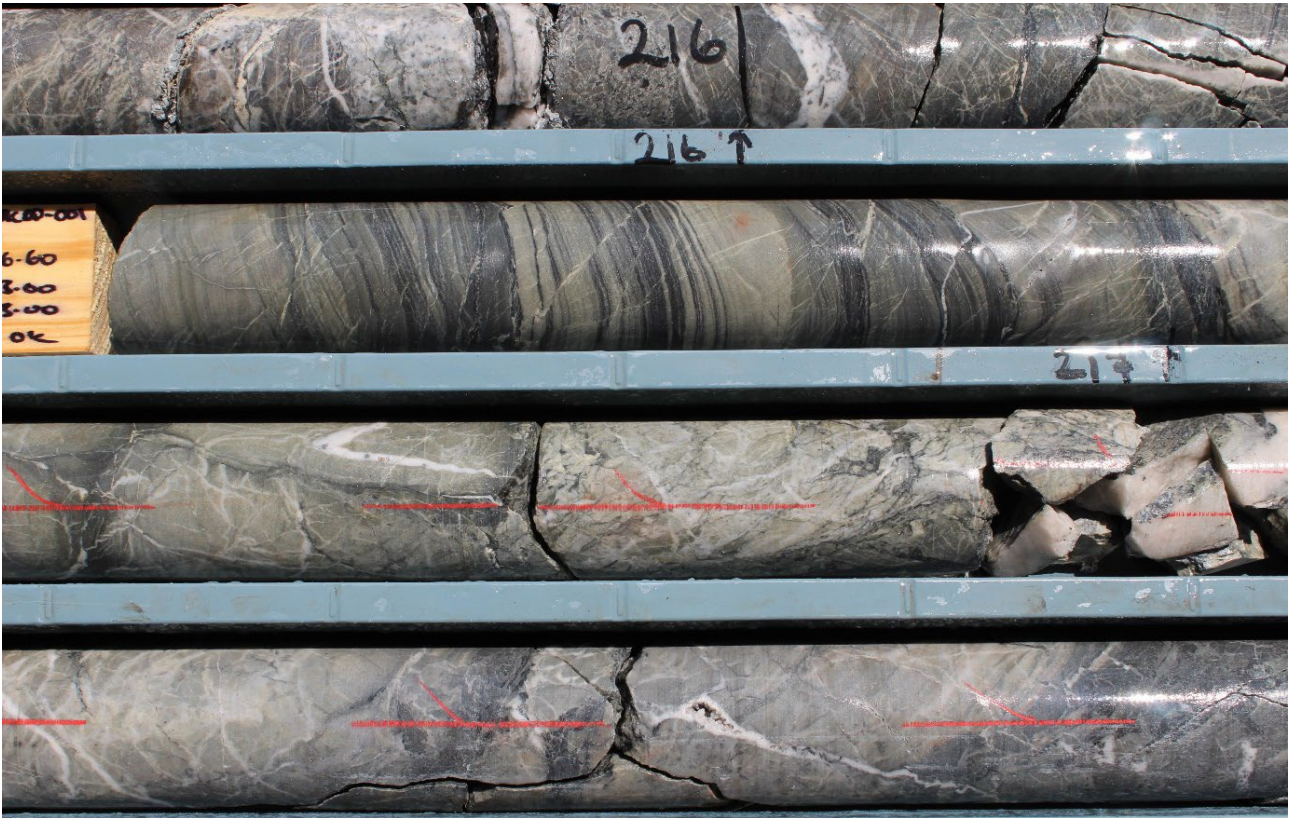
Figure 3: Intense texture destroying phyllic (silica-sericite) alteration present within WDRCDD001 from 215.62m to 218.93m.
