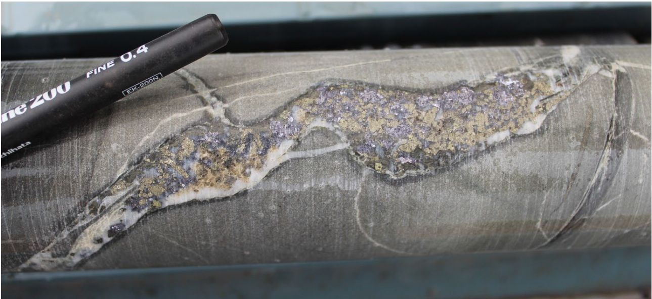
Figure 7: Stringer galena-quartz-pyrite-chalcopyrite-sphalerite vein in Clements Formation at 162.5m. Interpreted as representing a potential feeder zone for Browns Reef mineralisation. Refer to Table 1 for assay grades.
