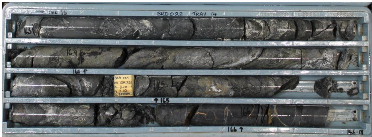
Figure 15: BRD022 main mineralised intersection between 163.6-166m down-hole. Intercepts included 2.4m @ 0.6g/t Au, 5g/t Ag, 1.9% Pb and 3.7% Zn including 0.5m @ 1.47g/t Au, 3.6g/t Ag, 1% Pb and 0.7% Zn from 164.5m.
