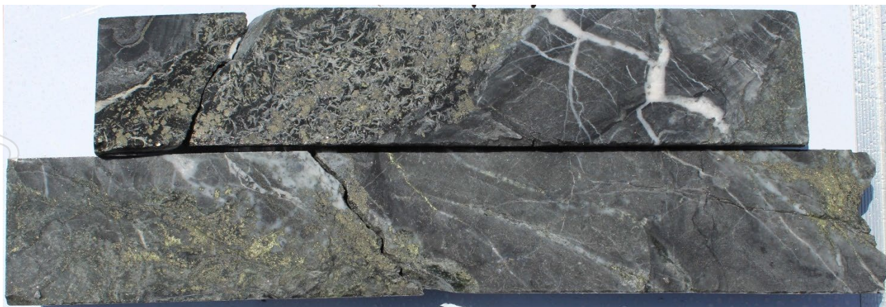
Figure 13: WDRCD001 291-291.7m pyrite, chalcopyrite and galena within the Preston Formation.
