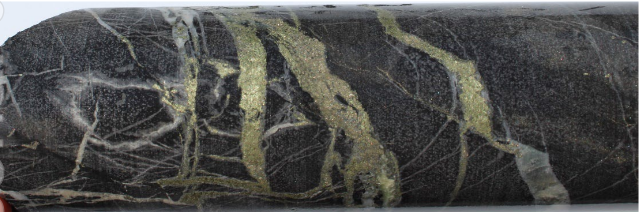
Figure 5: WDRCDD001 with chalcopyrite bearing breccia/vein fill zone intersected in the Clements Formation from 189.7m. Refer to Table 1 for assay grades.
