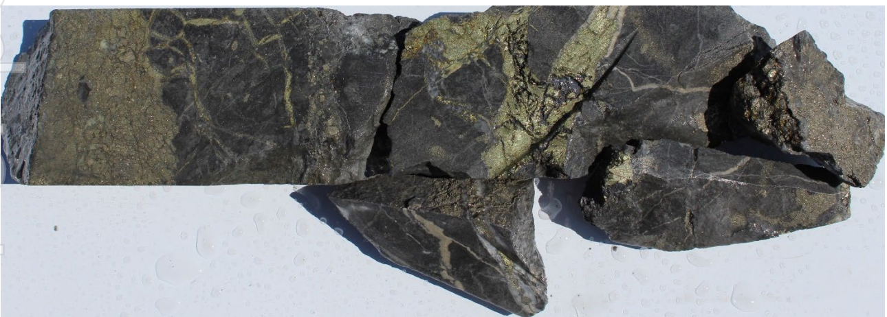
Figure 6: WDRCDD001 195.35-195.6m chalcopyrite, galena and pyrite breccia fill within the Clements Formation. Refer to Table 1 for assay grades.
