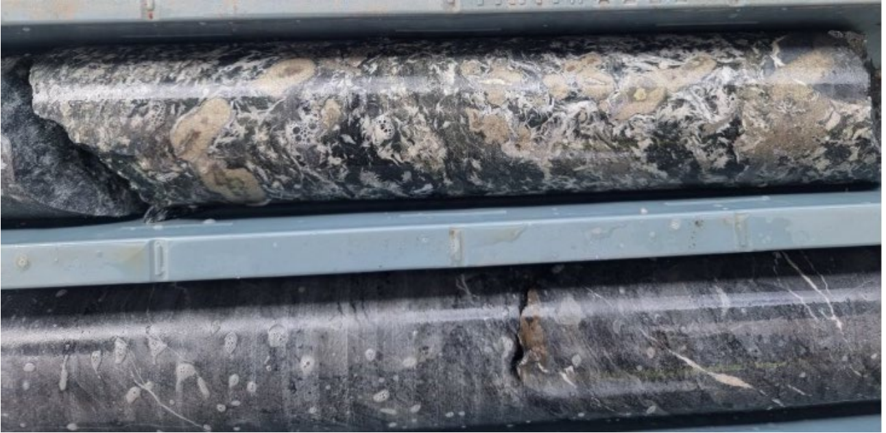
Figure 9: Possible dilation-zone replacement pyrite+chalcopyrite+(galena-sphalerite) in potentially ?fossiliferous sedimentary breccia in Devonian Preston Formation from 299.45m. Refer to Table 1 for assay grades.
