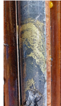
Figure 1. (a) Oxide, transitional and primary (fresh) resource estimation for the Tartana open pit using inverse distance estimation and a 0.2% Cu cutoff grade. (b) Primary copper mineralisation from drillhole D15.
