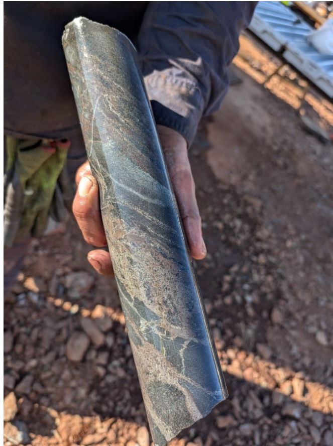
Figure 5: Sphalerite, galena and minor chalcopyrite in 24AED003
