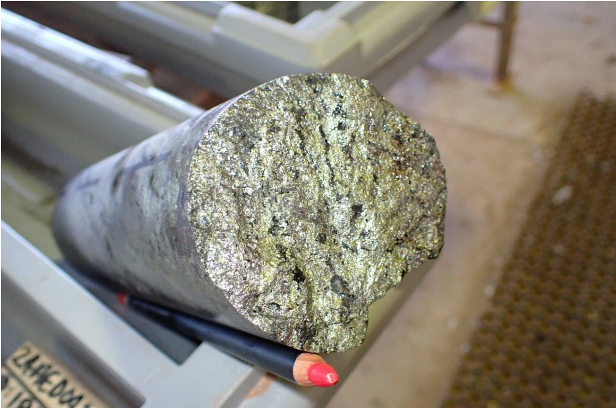
Figure 4: Massive sulphide mineralisation in 24AED002A
