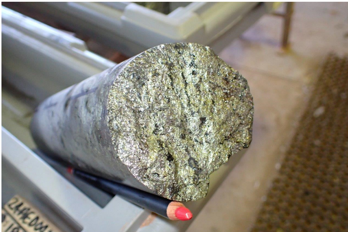
Figure 4: Massive sulphide mineralisation in 24AED002A
