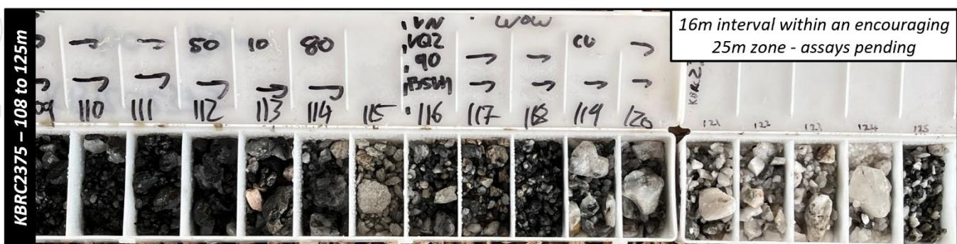
Figure 13: KBRC2375 chip tray 109 to 125m, 25m down dip of KBRC2302 (above) showing potential widening of sulphidic shale (pyrite, chalcopyrite, malachite, molybdenite & sphalerite), brecciated quartz and carbonates.
