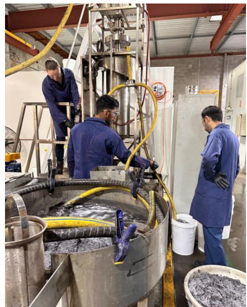
Figures 1 & 2: Pilot-scale flotation at the third-party testing facility in Australia
