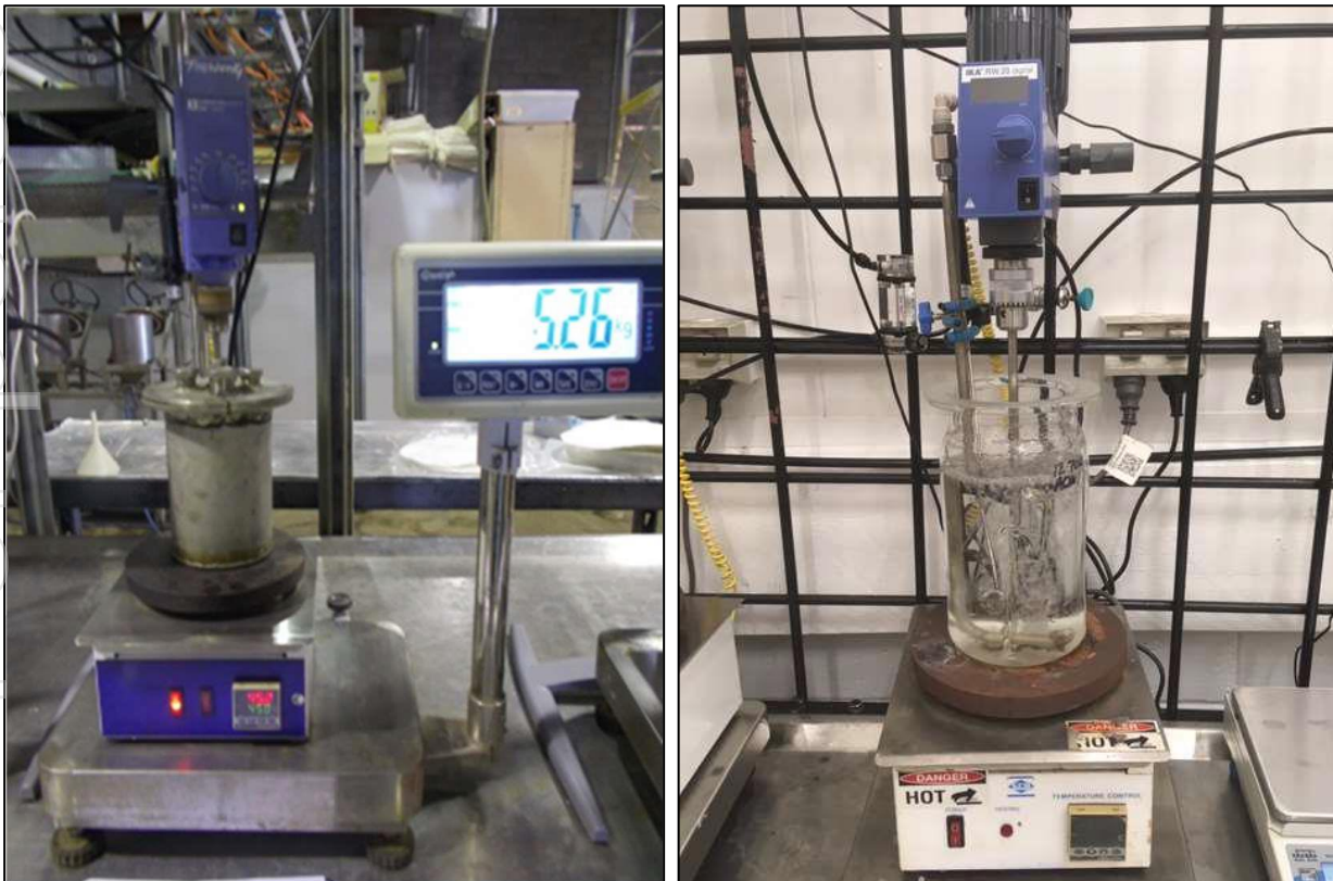
Figure 14. Montezuma Alkaline Sulphide Leaching and Air Oxidation Test Set Up
