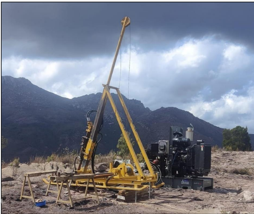
Figure 7. Montezuma Antimony Project diamond drill rig suitable for surface and underground drilling – one of multiple pieces of equipment being acquired
