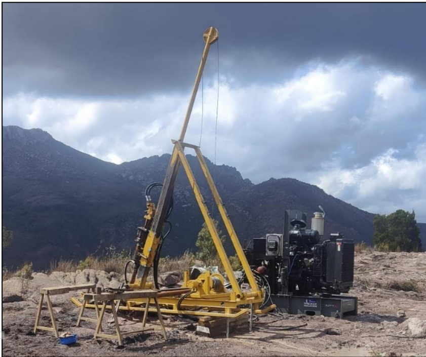
Figure 7. Montezuma Antimony Project diamond drill rig suitable for surface and underground drilling – one of multiple pieces of equipment being acquired
