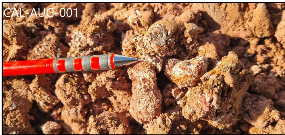
Figure 3 - CLD-AUG-001 interval from 9.00 to 10.00 metres – 7,099ppm TREO clay zone with disseminated kaolinite
