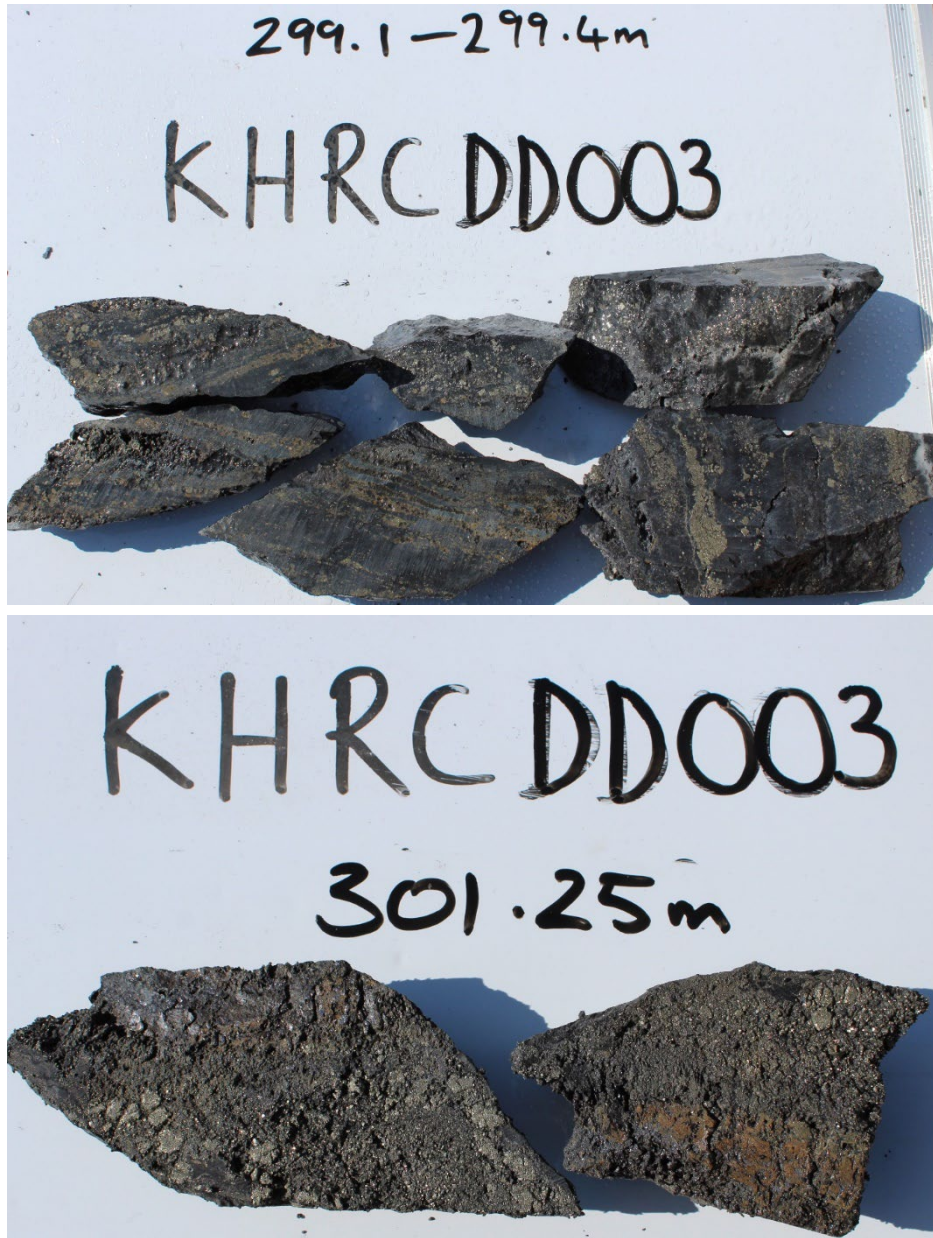
Figure 5: Laminated semi-massive to massive galena-pyrite-sphalerite in hole KHRCD003, Preston Formation. Refer to Table 1 for assay grades.
