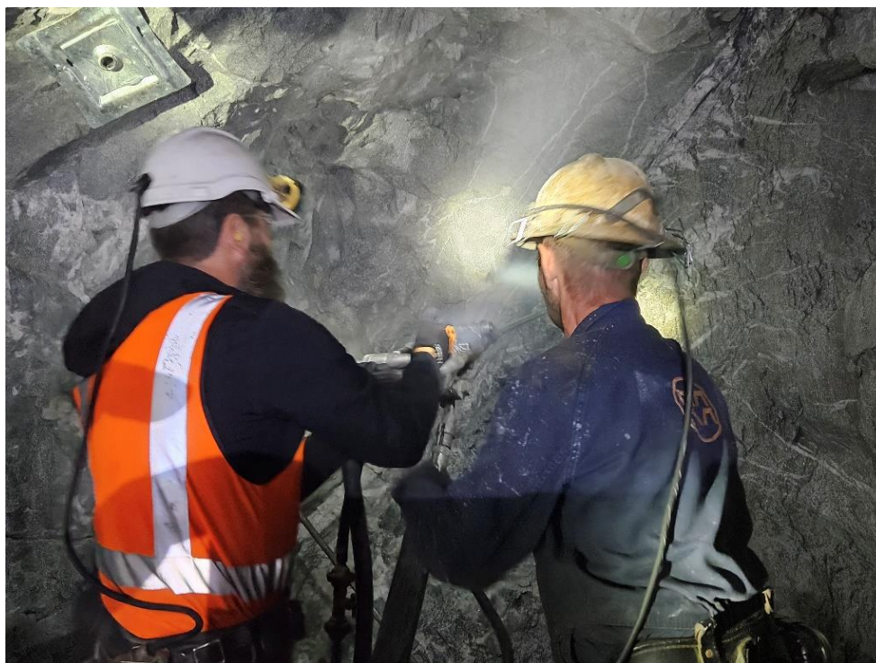
Figure 7: High grade airleg mining on the Tasma Reef.
