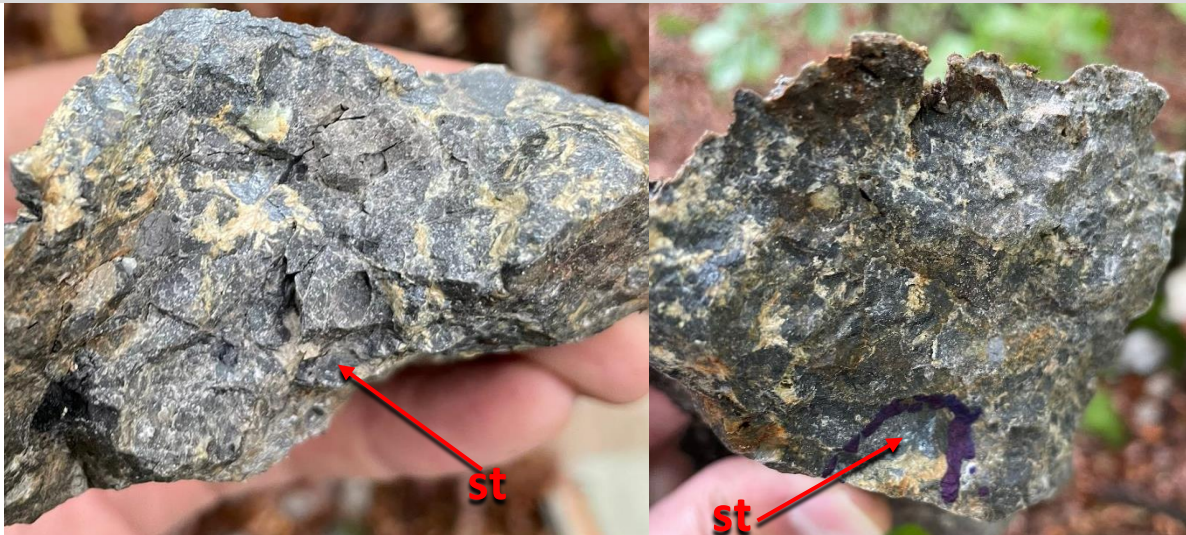
Figure 1 Photographs of recent Bindi samples at Kreva 1 (left) Sample DM014022 displaying 5-20% massive stibnite (antimony sulphide mineral; st ); (right) Sample DM014024 displaying 1-2% disseminated stibnite ( st )
