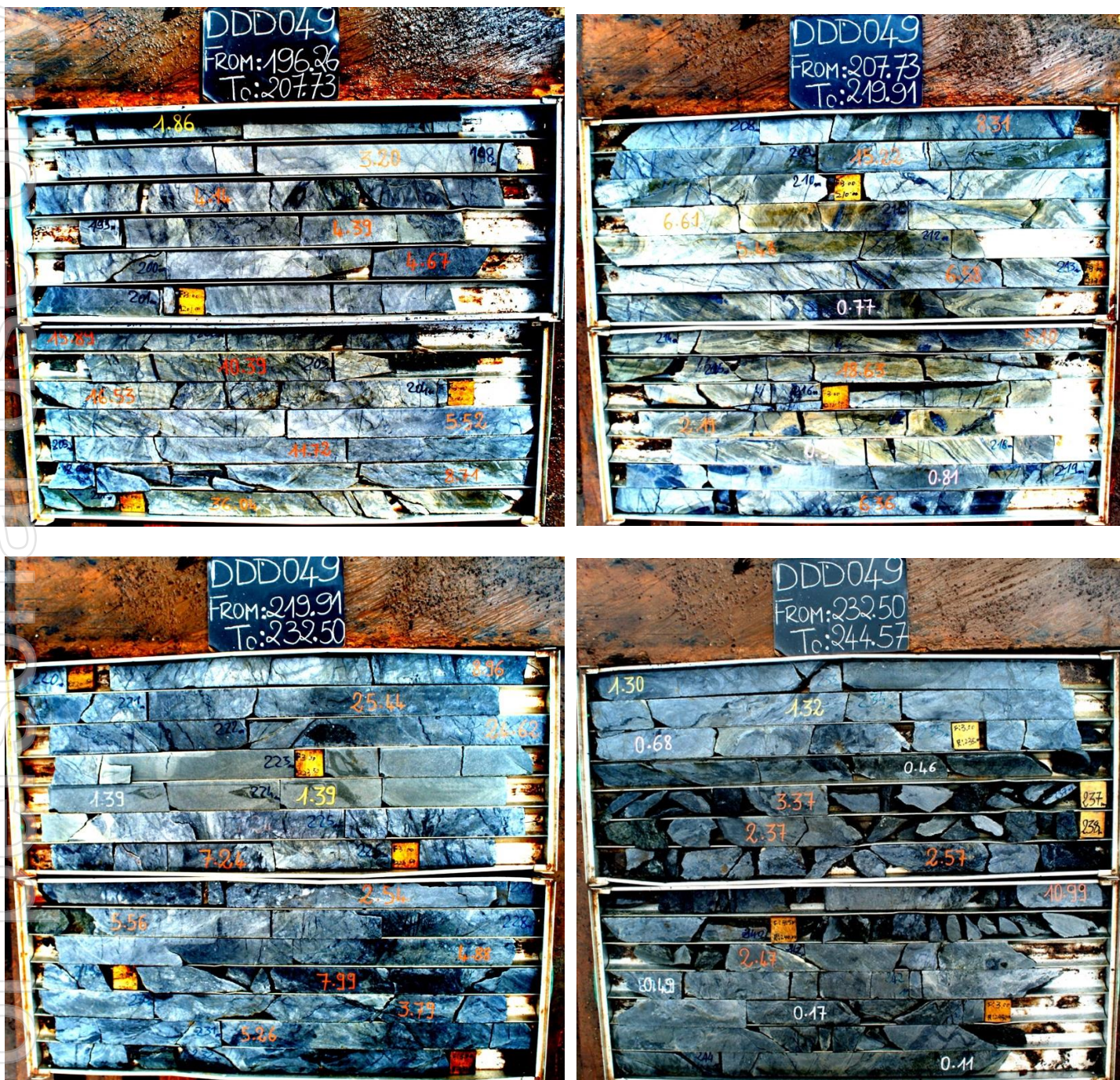
Figure 2: Photographs of the intersection of 65m @ 5.6 g/t of gold from 177m of the diamond drill core from drill hole DDD049.
