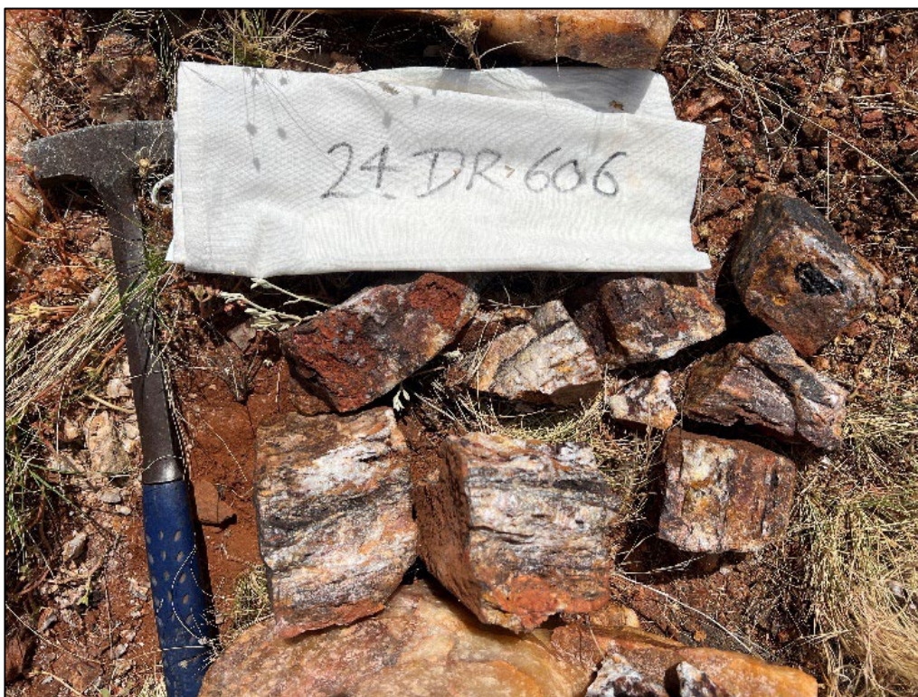
Figure 8. Oxide-sheathed quartz vein sample from the Thylacine Prospect (assays pending)
