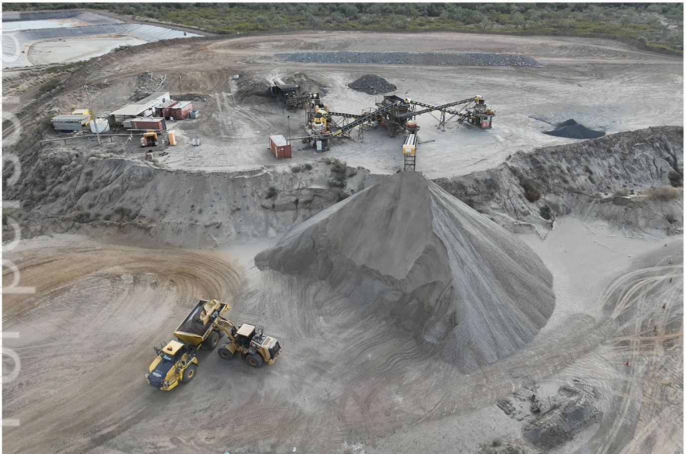
Figure 1. Recovery of crushed stockpiles for transport to the leach pad.
