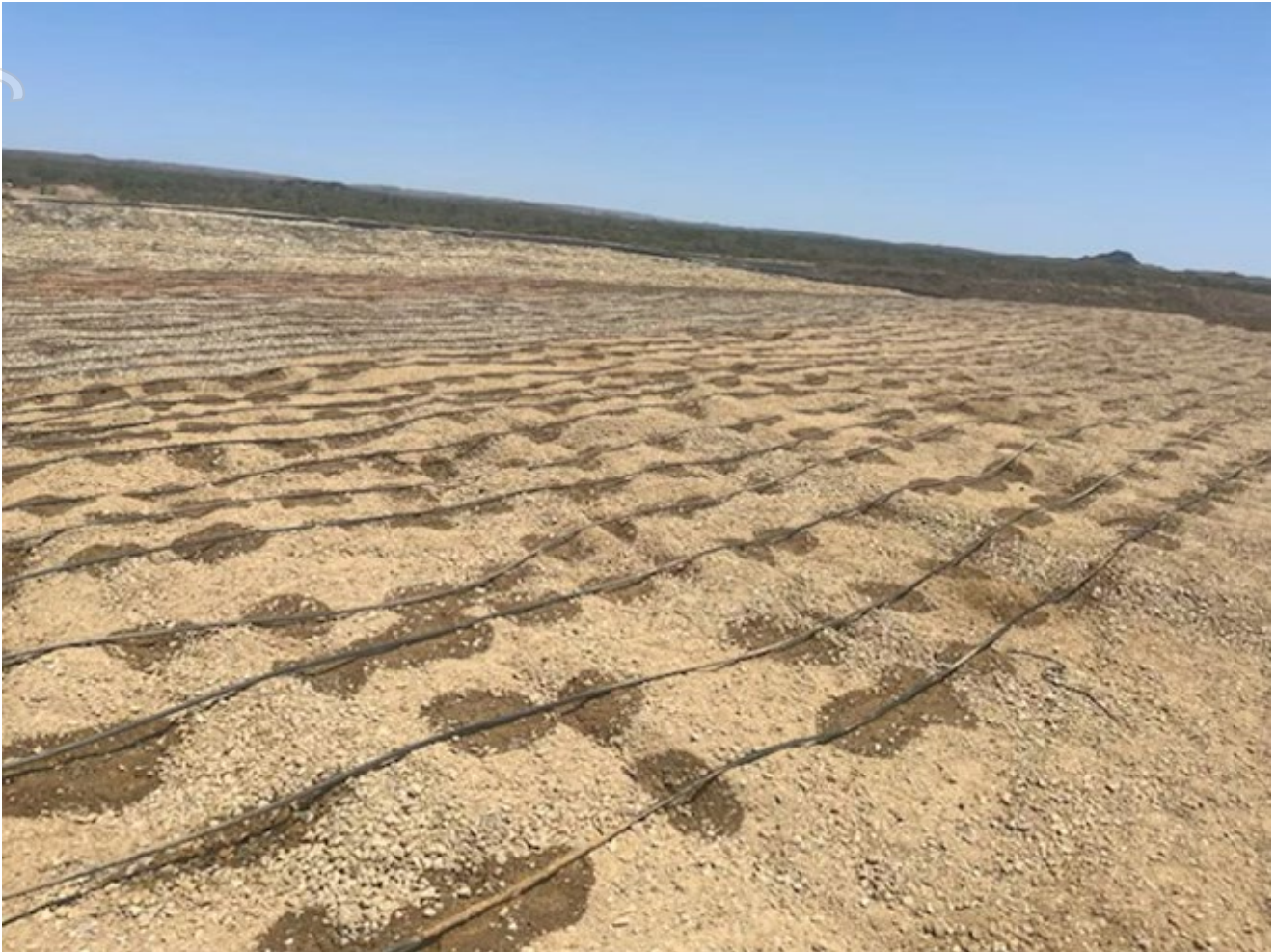
Figure 2. Leach pad 5 under irrigation on 8 October 2024.
