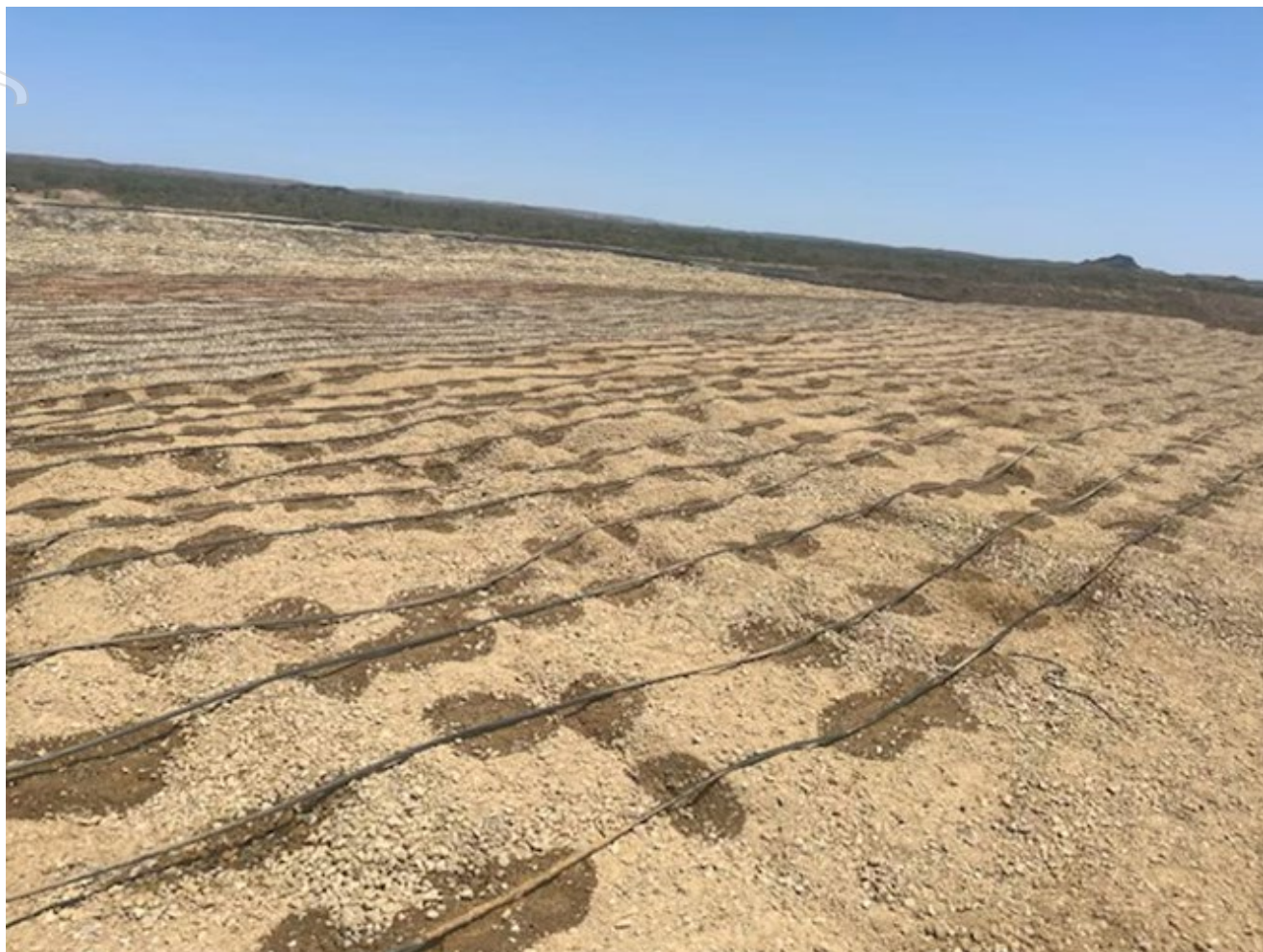
Figure 2. Leach pad 5 under irrigation on 8 October 2024.
