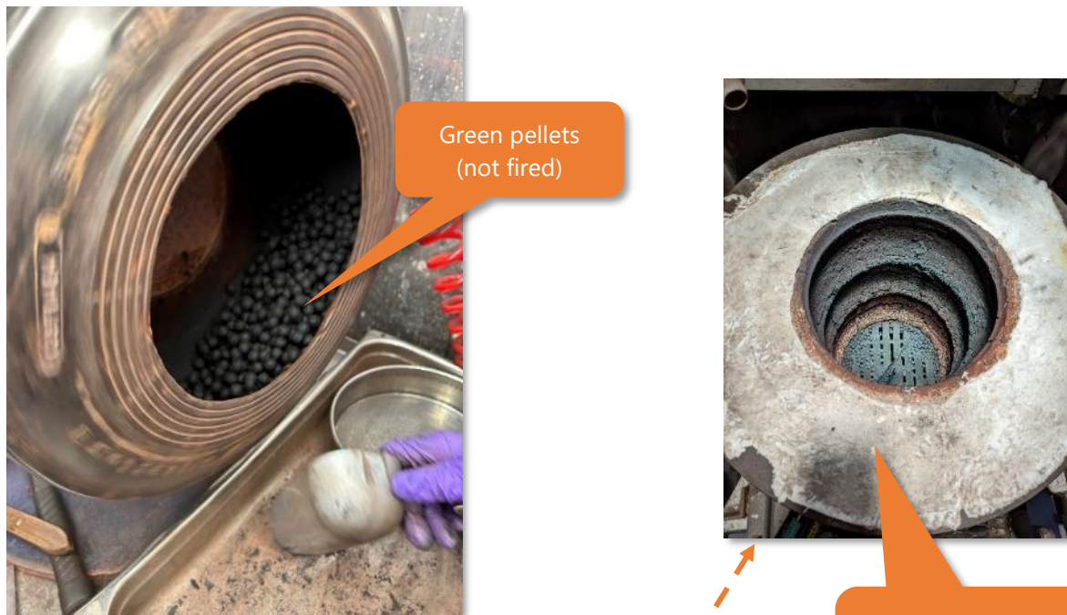
Figure 2: Photo of green balls being produced from iron bear concentrate
