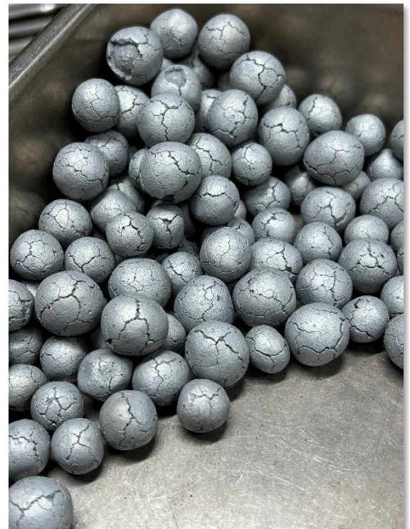
Figure 7: Pellets after Linder metallisation / reduction
