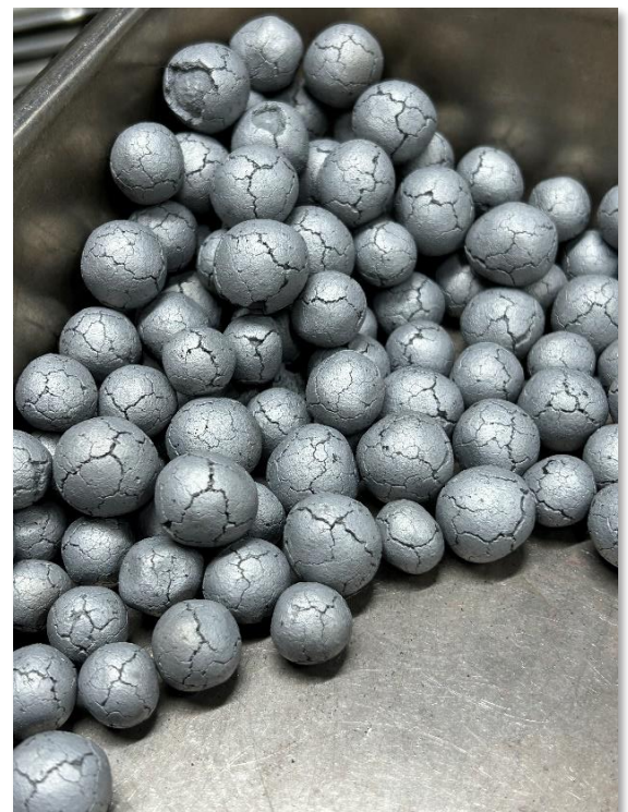
Figure 7: Pellets after Linder metallisation / reduction
