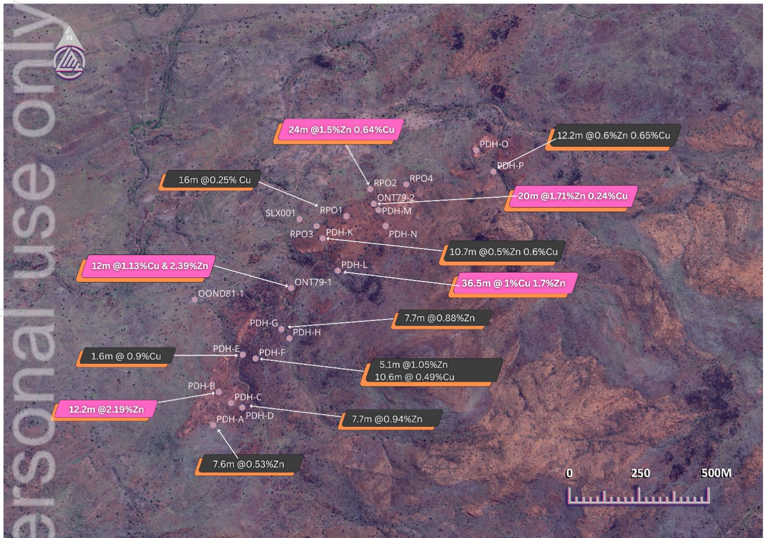
Figure 4. Oonagalabi historic drilling showing mineralisation over a 1.5km strike. Opportunities to expand mineralisation exist at depth (shallow historic drilling) and with testing blind IP chargeability anomalies on the eastern limb of the anticline.
