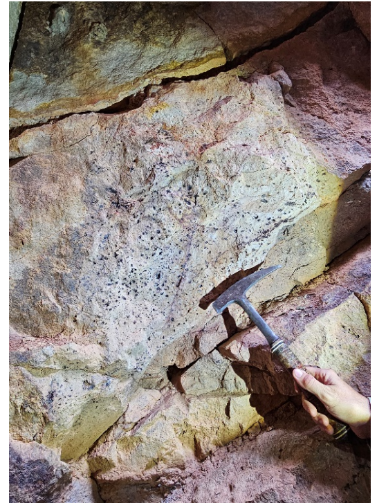
Wall Rock inside Daisy Bell - showing disseminated and massive cassiterite crystals, rock XRF tests 7% tin after milling then scanning.
