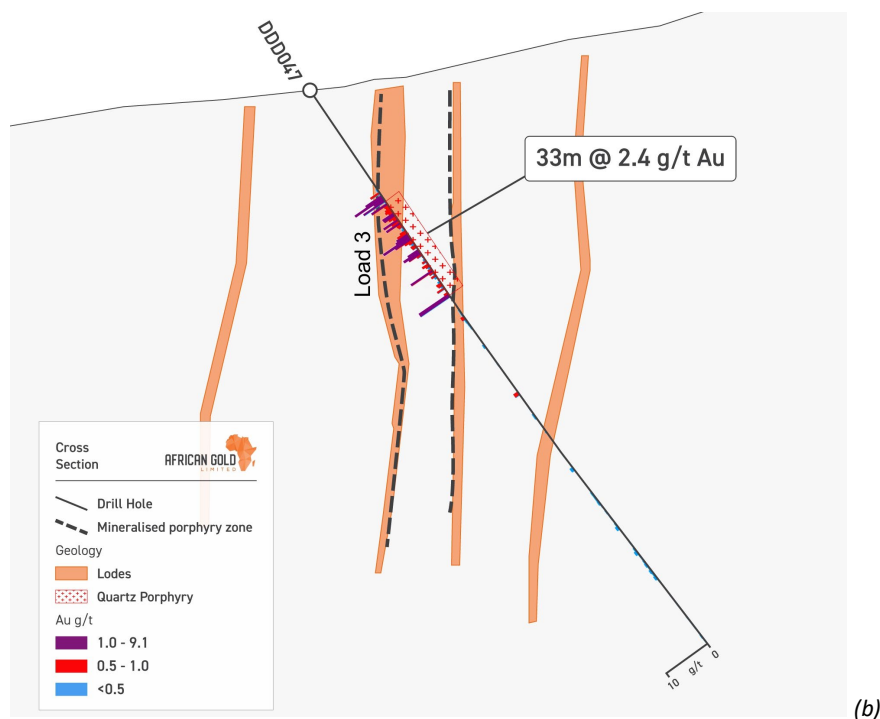
Figure 3: Details of the drillhole DDD047: (a) geological map of the DDD047 drillhole area, modified after Equigold 2010 prospecting data; (b) Cross section of prospect drawn through the drill hole DDD047.
