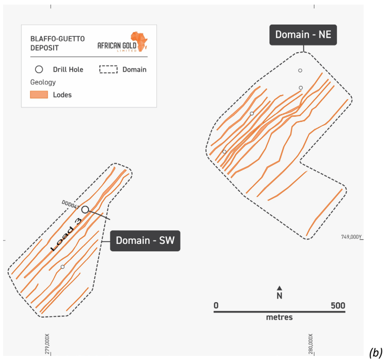
Figure 1: Map of the Blaffo Guetto prospect showing location of the new drillholes (the collars are shown as the dots). Trace of the DDD047 is shown for the reference; (a) gold lodes projected on the surface and shown on the geological map; (b) gold lodes.
