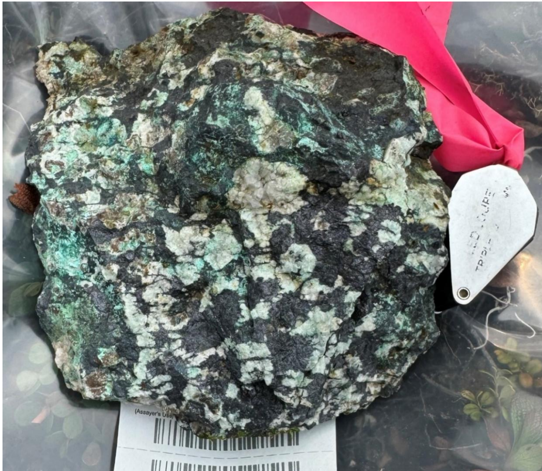
Figure 6: Photograph of sample location F005982 from the PAT target which returned 20.1% Cu and 18g/t Ag.
