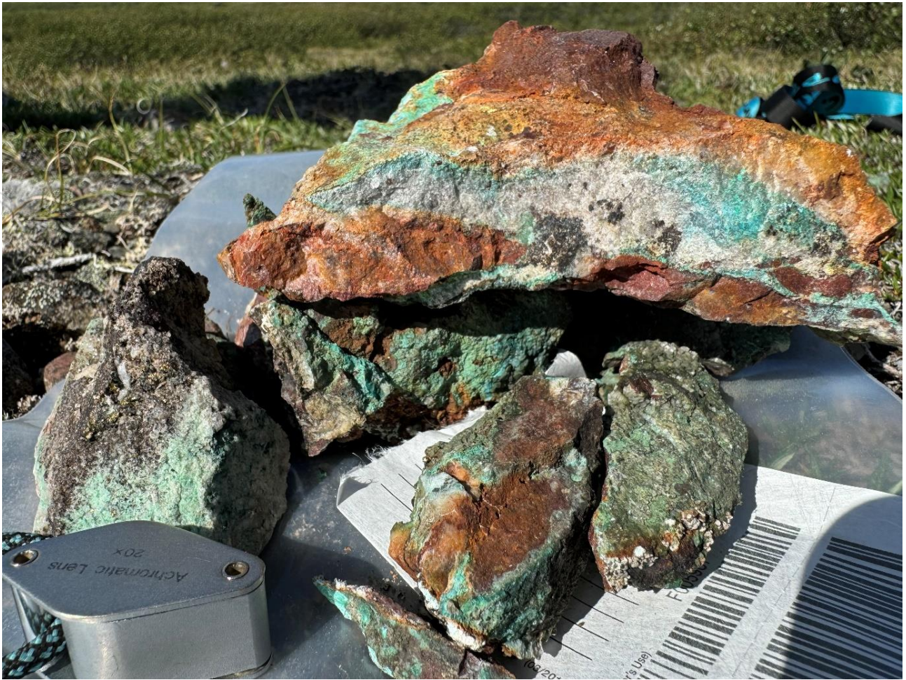
Figure 13: Photograph of sample F005987 from the CALMAL target adjacent to the Hulk District, showing chalcopyrite-malachite mineralisation within a quartz sandstone and quartz vein which returned 1.65% Cu .
