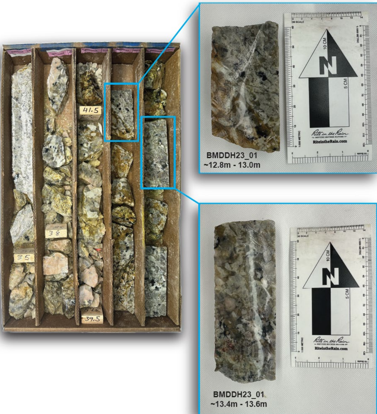
Figure 2: Black Mountain pegmatite intersection in BMDDH23_01 from 10.5m (34.5ft.) to 13.7m (45ft.) showing some of the spodumene mineralization (See Chariot's ASX Announcement dated 2 February 2024)
