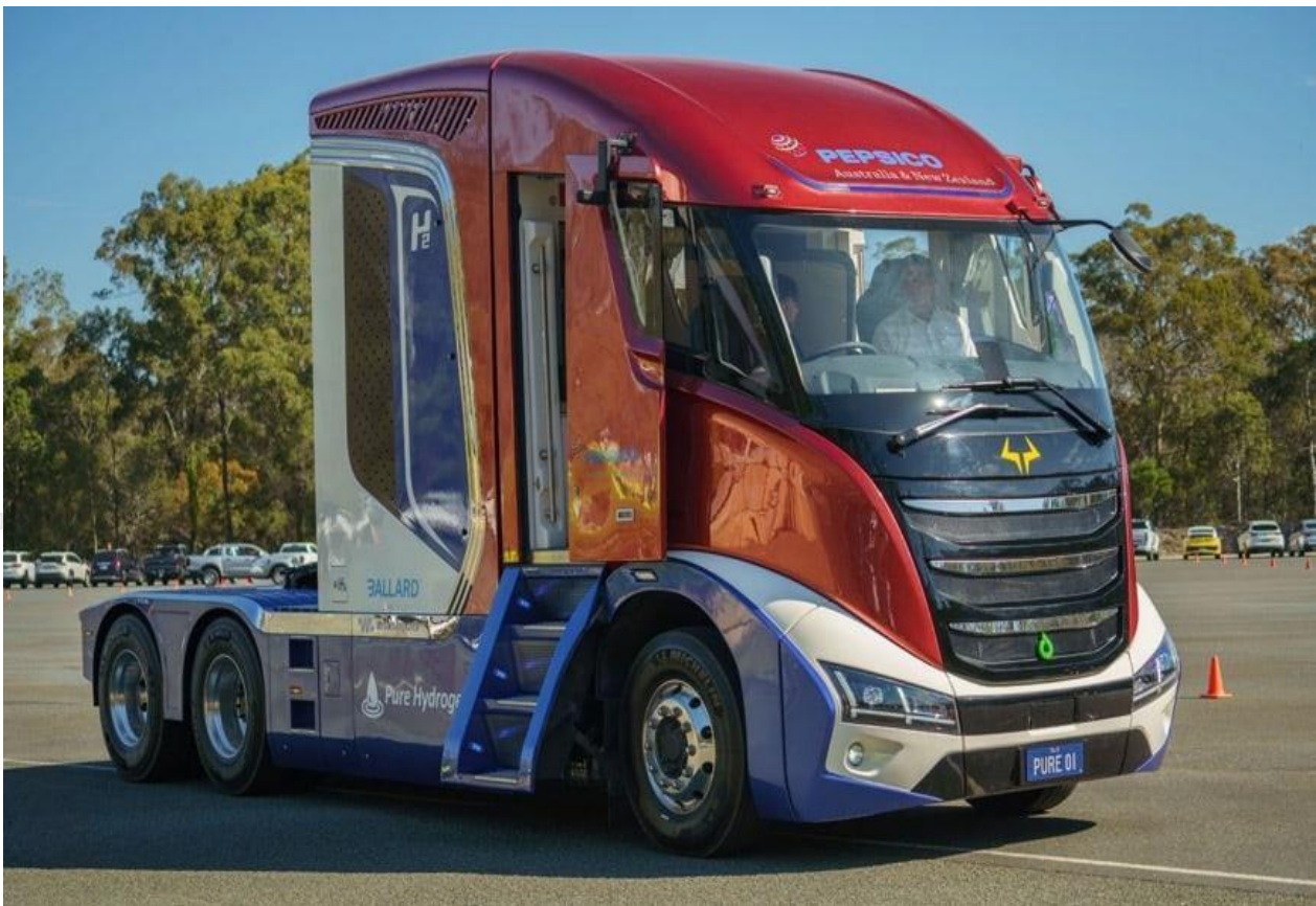
The 'Taurus' hydrogen-powered Prime Mover
