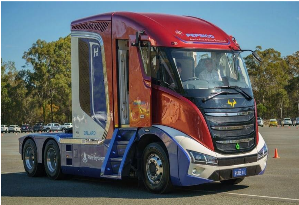
The 'Taurus' hydrogen-powered Prime Mover
