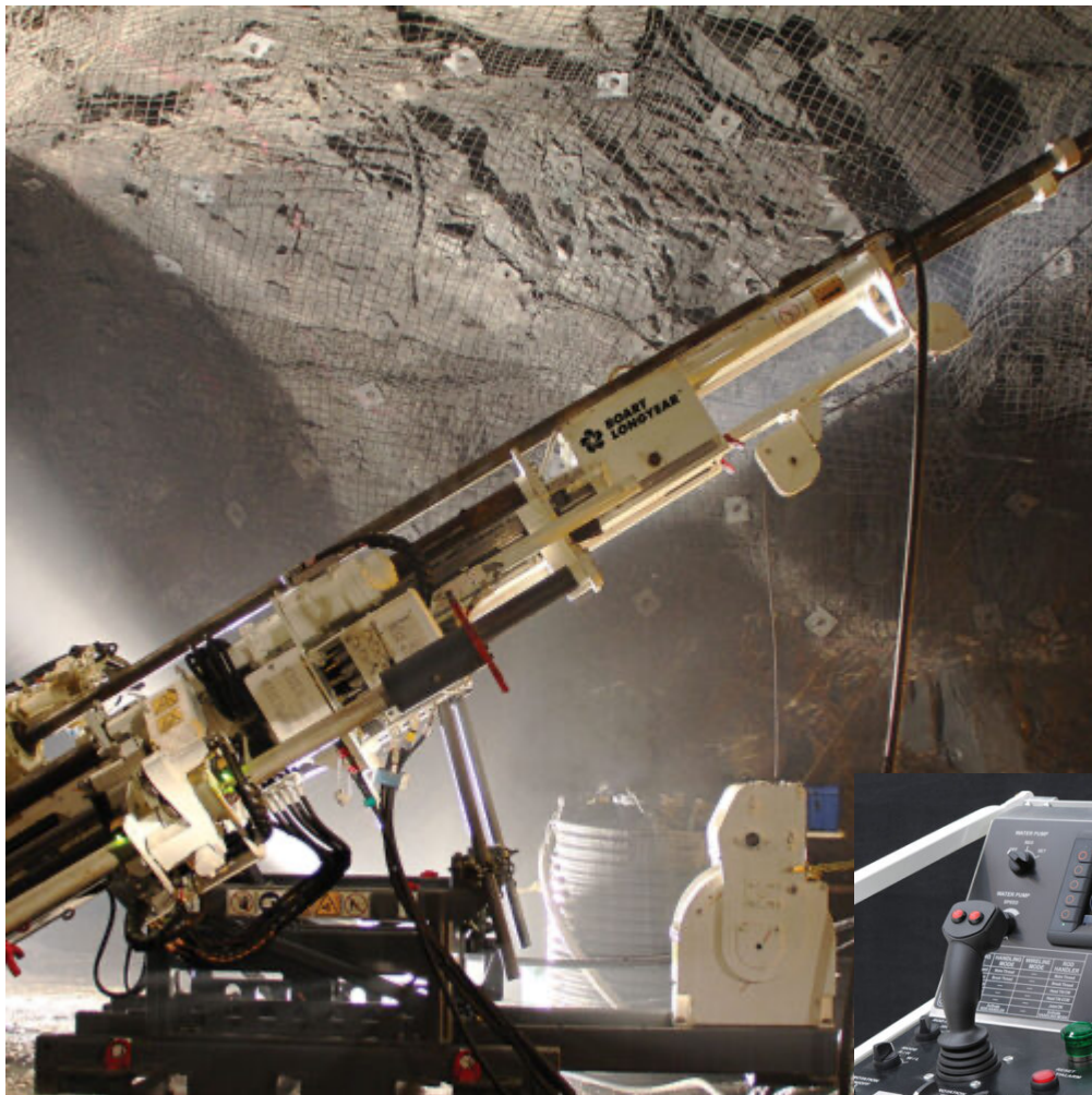
Figure 1: LM 90 Underground Drill Rig with Rod handler
