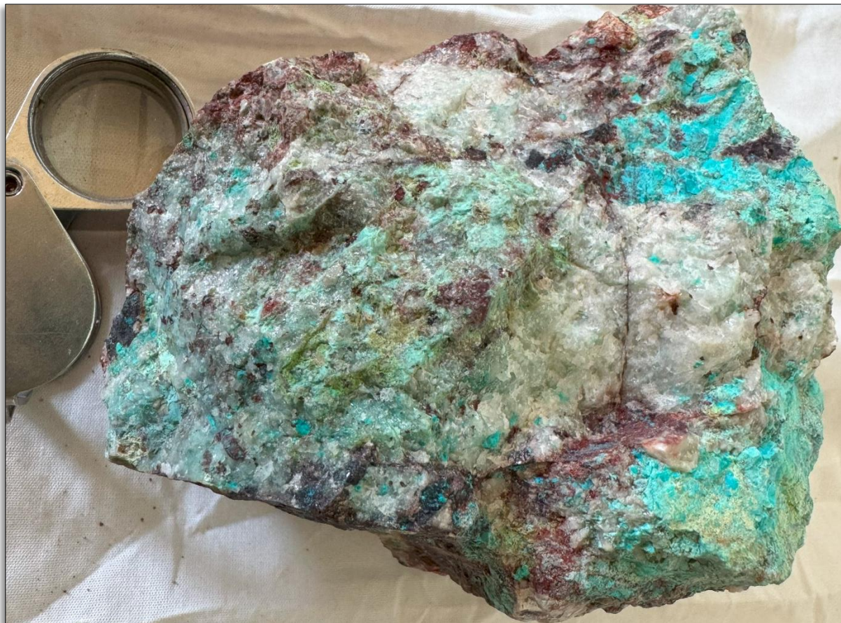
Figure 3: 24PRL002. 930 g/t Ag, 2.37% Cu. Quartz vein with iron oxides, copper carbonate within granodiorite host rock.
