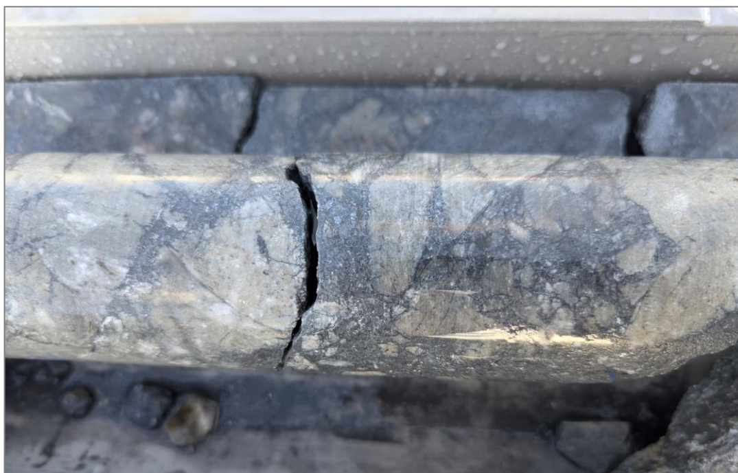
Figure 5: Core photo of the high-grade Sb interval in RDRC067 highlighting brecciated ultramafic at 239.4m. Refer ASX Release 26 August for full context)
