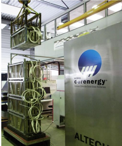
Photo: Prototype 60 kWh battery being assembled and tested at Fraunhofer IKTS laboratory
