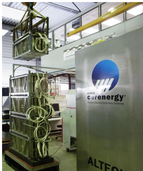
Photo: Prototype 60 KWh battery being assembled and tested at Fraunhofer IKTS laboratory
