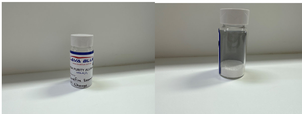
Plates 1,2: Some of the first 4N 9.99% HPA generated by Lava Blue from the Company's Victory Bore deposit
