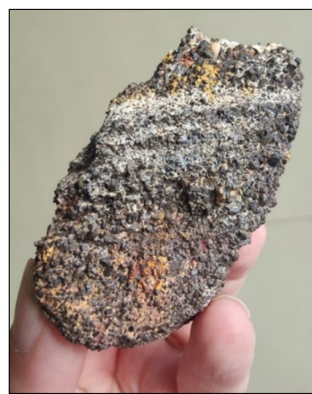
Photo – Left – Typical outcrop of HMS titanium ore (dark minerals) in white silts. Right – high-grade ores (>30% TiO 2 ) from the Rosewood Prospect. The brown-black minerals are the Titanium-bearing mineral ores comprising ilmenite, leucoxene and rutile.
