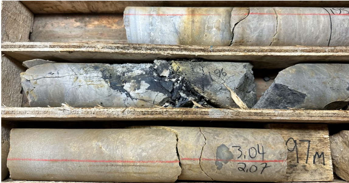
Figure 17: Chalcocite (dark grey) fracture fill in drill hole ST24-02 from approximately 196m downhole.
