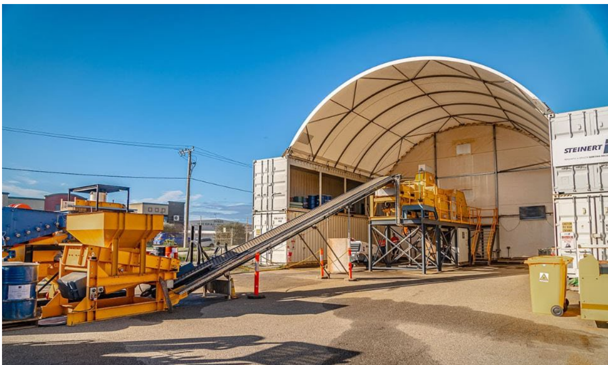
Figure 6: Photo of a Steinert KSS KLI XT ore sorter and feed bin. Source – Steinert.
