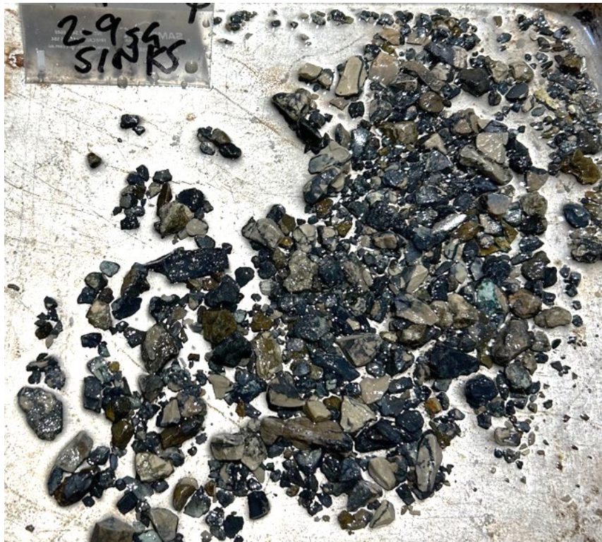
Figure 8: Photo of a DMS Viking (IPJ) DSO product on -11.2/+2.46mm ore-grade composite material. The density cut is at a 2.9 SG and returned a grade of 51.3% Cu. Note the dark grey/black particles which are chalcocite (copper sulphide), and light grey host rocks (dolomite).
