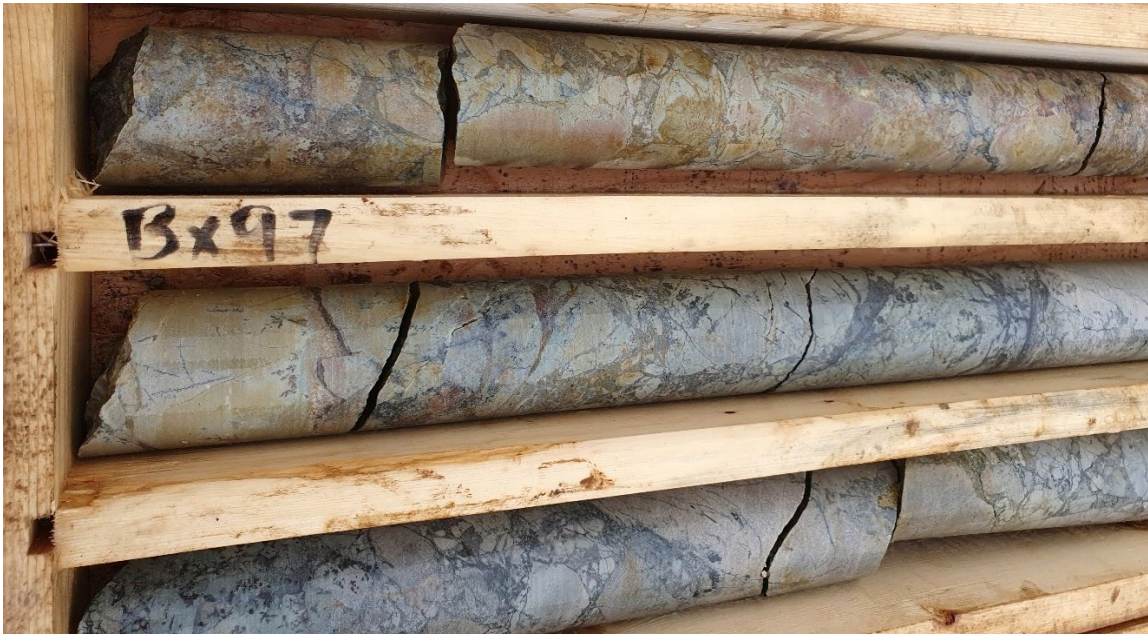
Figure 15: Drill core from ST24-01 from approximately 315.4 – 318m downhole. Dense veins and breccia of visible chalcocite (copper sulphide) can be seen as dark sooty grey, within light grey/mustard dolomite host rocks. This interval also contains blebs of native copper (brassy gold).
