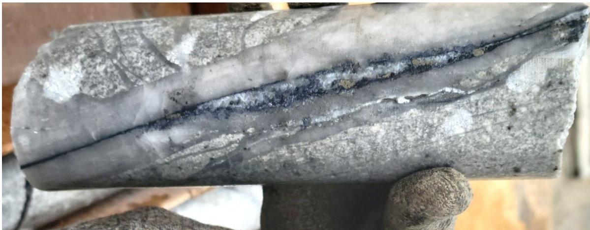
Figure 24: Photo of molybdenite + quartz + pyrite veining within quartz monzonite porphyry stock in drill hole WD22-04 (interval 640.66-642.18m downhole @ 0.22% Mo). 4
