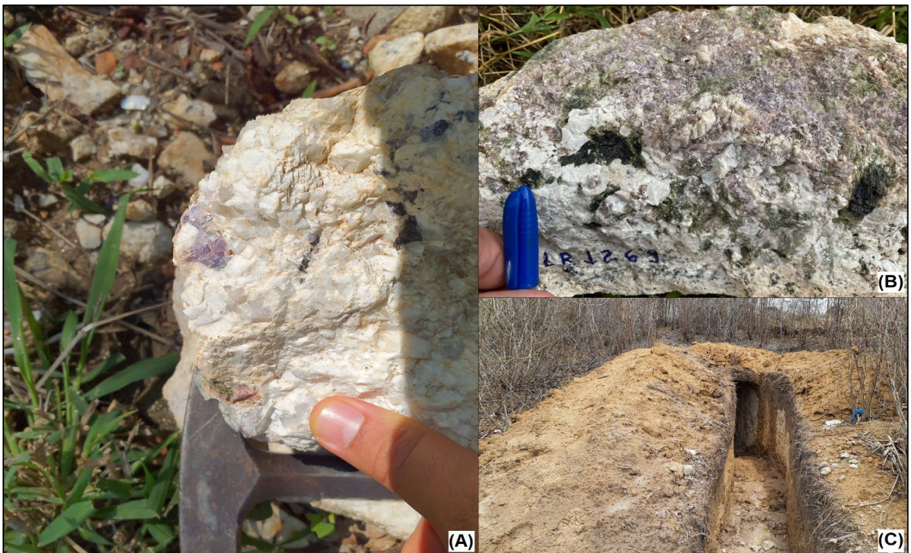
Figure 2: (A) Photograph of sample BLR237 showing lepidolite minerals (purple) within pegmatite sample (B) Photograph of sample VLR1269 showing lepidolite minerals (purple) within pegmatite sample (C) Photographic example of workings located within the larger Caraibas tenement area (805118mE, 8193908mN)
