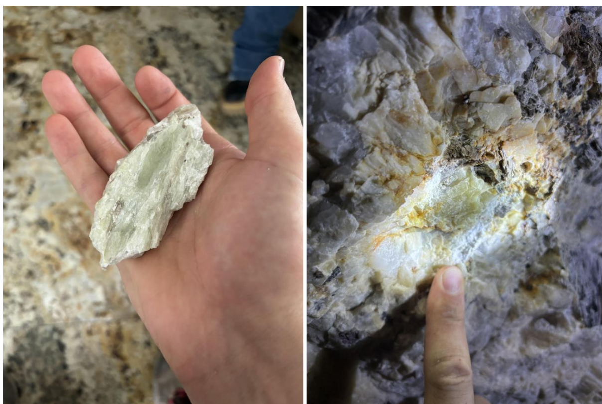
Coarse spodumene (Sample ID: IZAPEC006) (left) & in-situ spodumene located within artisanal mine (Garimpo 2 - right) from Isabella Project, license 830167/2013, (Refer to ASX announcement 24th July 2024, for rock descriptions)
