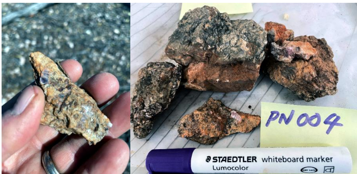
Figure 8: Rock chip PN004 showing coarse lepidolite crystals in pegmatite which returned 0.45% Li 2 O
