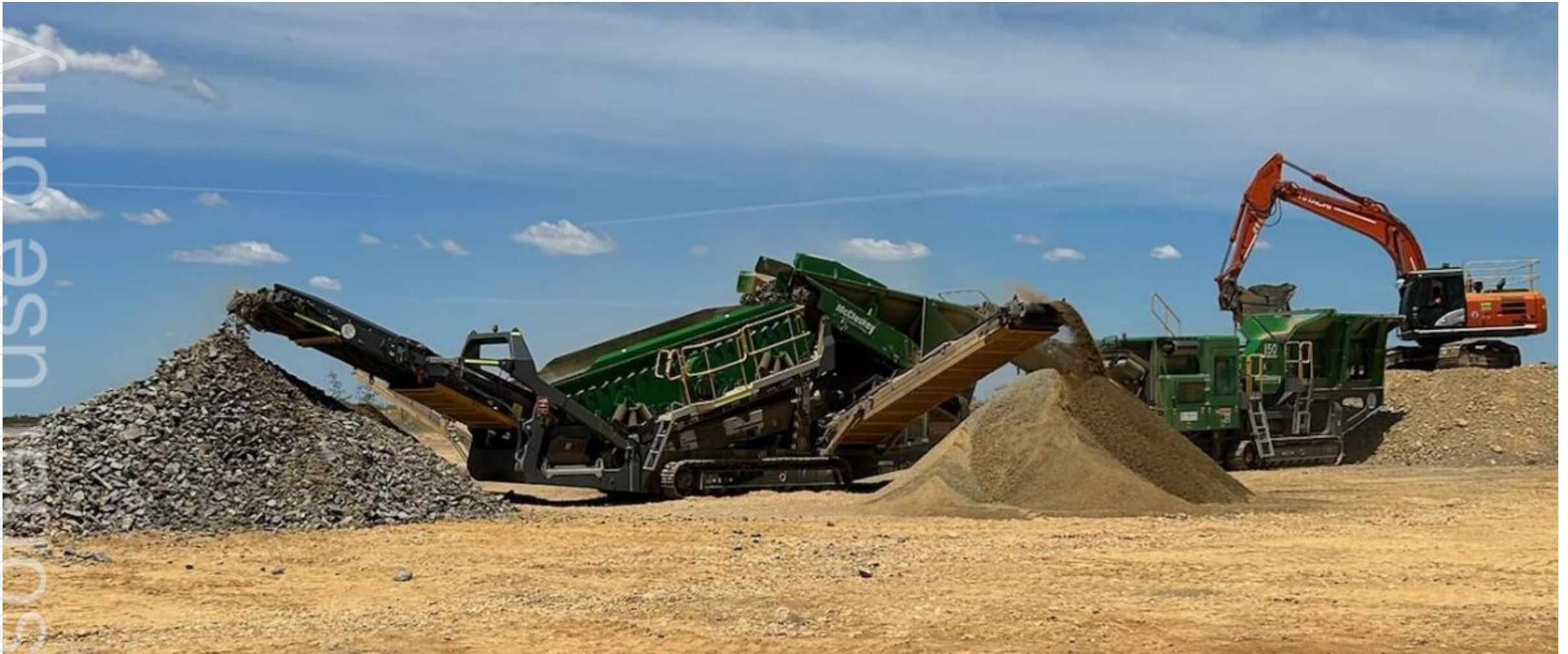
Photo of the McCoskey R230 'reclaimer' mobile screening plant at Mt Boppy.
