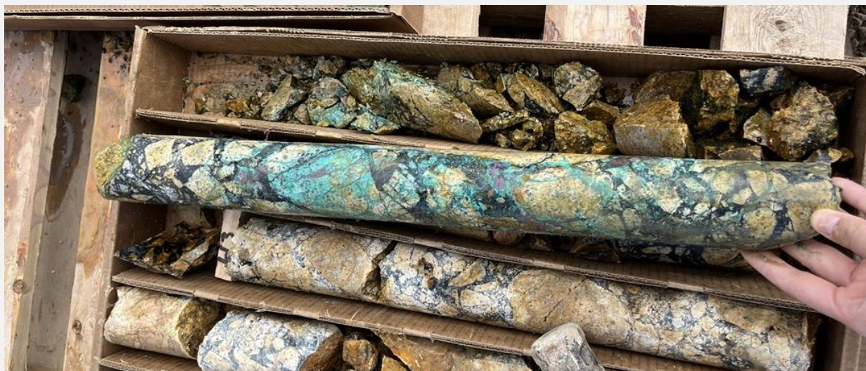
Figure 1: High grade copper mineralisation in tourmaline breccia which contains pXRF grades up to 45.5% copper within the interval 14-16m down hole NY2024-DDH2
