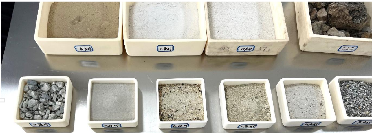
Figure 12: Various Spodumene Concentrates from around the world showing various particle sizing and grades
