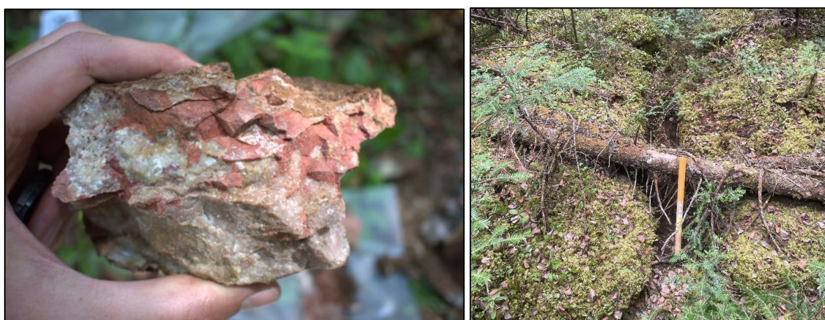
Figure 2. (Left) REE mineralisation (red mineral) 3.6% TREO and 0.5% Nb 2 O 5 from the Blue Jay prospect and (right) historical trench at Goldfinch with results of 7.6m @ 0.3% Nb 2 O 5 and grabs up to 1.82 % Nb 2 O 5 with resampling returning 0.35% TREO, 0.2% Nb 2 O 5 and 130 ppm Sc 2 O 3 .
