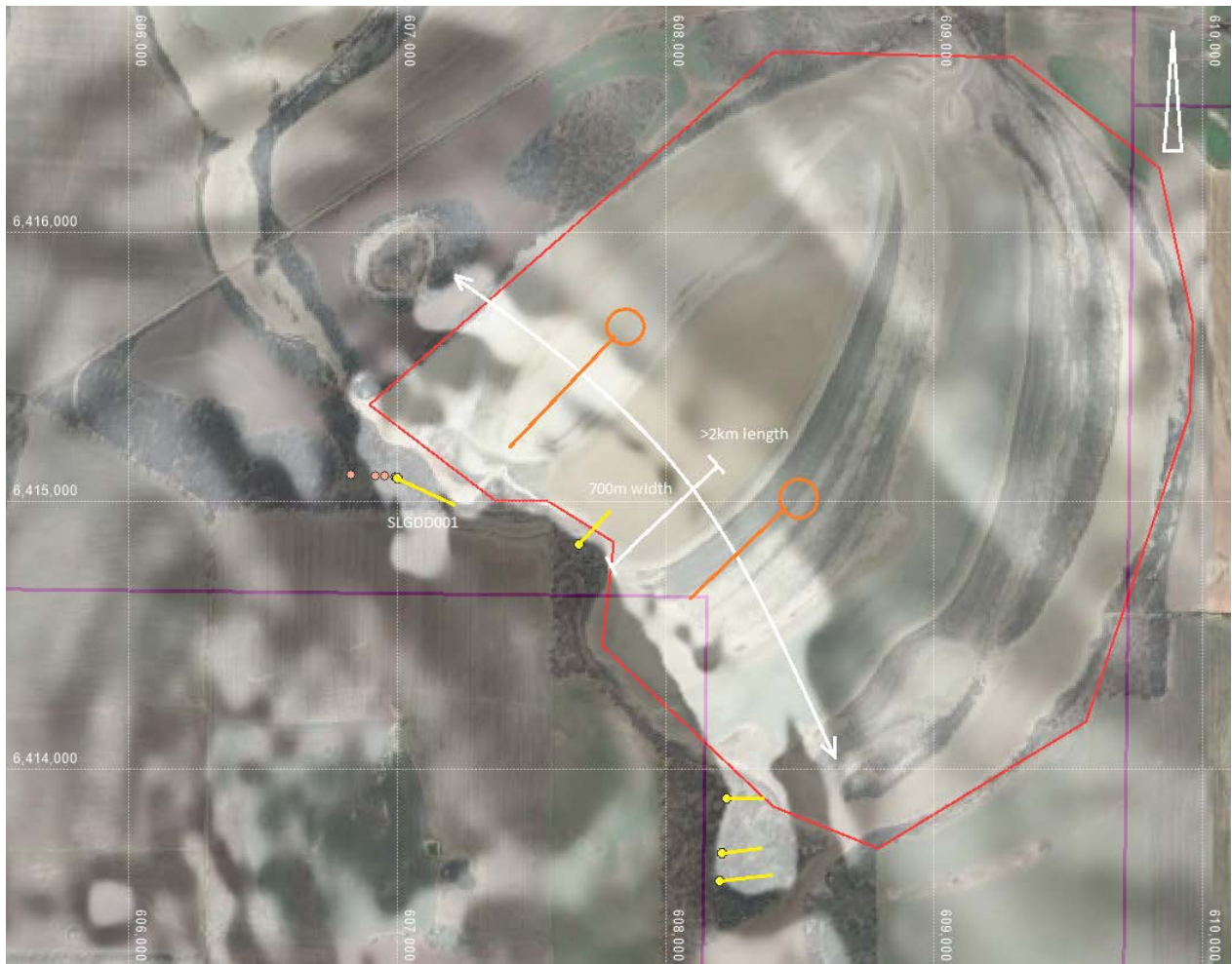
Figure 4: Plan view of 1VD magnetic signature representing the >2km long, 700m wide ultramafic sequence overlain by aerial photography highlighting the salt lake, with Reserve 18455 (Lot 225568) highlighted in red. Sultan's 2022 aircore collars are marked in orange, and previous diamond drilling traces in yellow, with recent SLGDD001 named. Orange circles and traces indicate possible drilling collar positions to test the layered intrusion from the salt lake surface.
