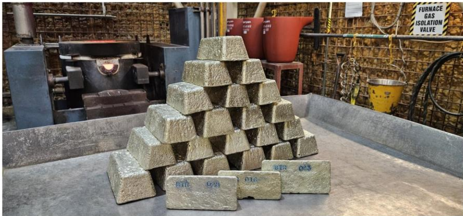
Figure 14 - Shipment 2: Gold doré bars BTR005 – BTR016 (poured on 9/3/24) and BTR017 – BTR028 (poured 12/3/24)
