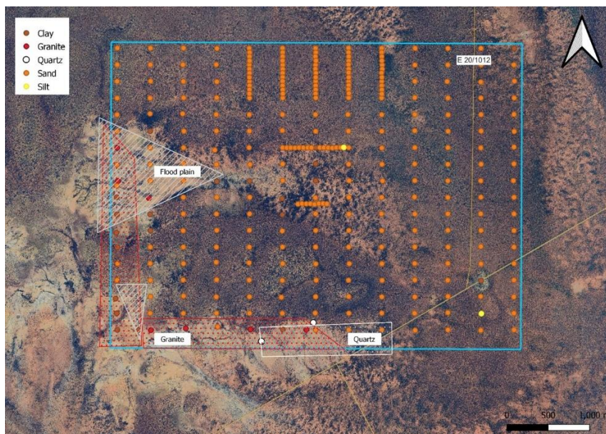
Fig 1, Soil Sample Survey over Google Image, showing sample soil types
