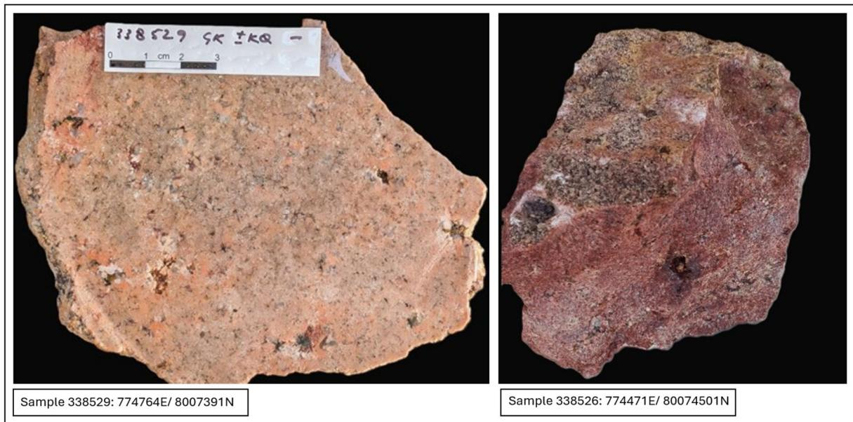
**Plate 2:** **Sample 338529:** Aplite “clasts” isolated by coarser feldspar, quartz and miarolitic cavities. The distribution of the quartz + oxidized sulphide miarolitic demonstrate in detail, the aplite magma was brecciated whilst still in a “mushy” magmatic state.
