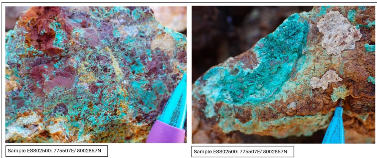
Plate 4: Sample ESS02500: High grade copper oxide mineralisation as cuprite (red-brown), malachite and chrysocolla. Located in the central-southern sector of the Yataga Valley Copper Prospect and shows quartz + sericite + sulphides in altered granodiorite.
