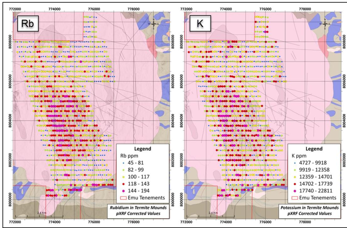
**Figure 5:** pXRF geochemistry for Potassium (K) and Rubidium (Rb) characteristic of highly fractionated granitoid intrusive rocks and potassic hydrothermal alteration indicative of porphyry copper scale processes pervading the Yataga Igneous Complex. A 4km long x 2.5 km wide elliptical anomaly is centered on central “core” zone, with the Yataga Valley Prospect being the dominant K & Rb anomaly identified to date.
