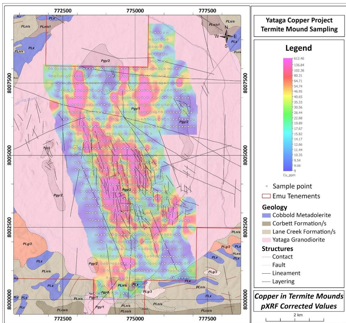
**Figure 1:** The termite mound geochemical sampling programme grid with Copper (Cu) heat map overlying geology. The main Cu-zones of Fiery Creek Prospect and Yataga Valley Prospect are clearly defined. (See also Figure 4.)
