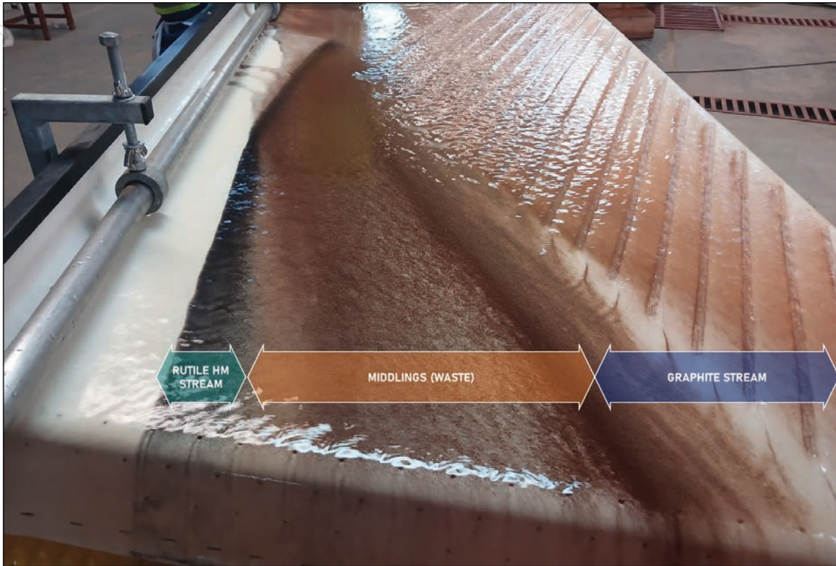
Figure 9: Holman Wilfley 2000 wet shaking table in action demonstrating clear separation between Rutile HM, waste and Graphite
