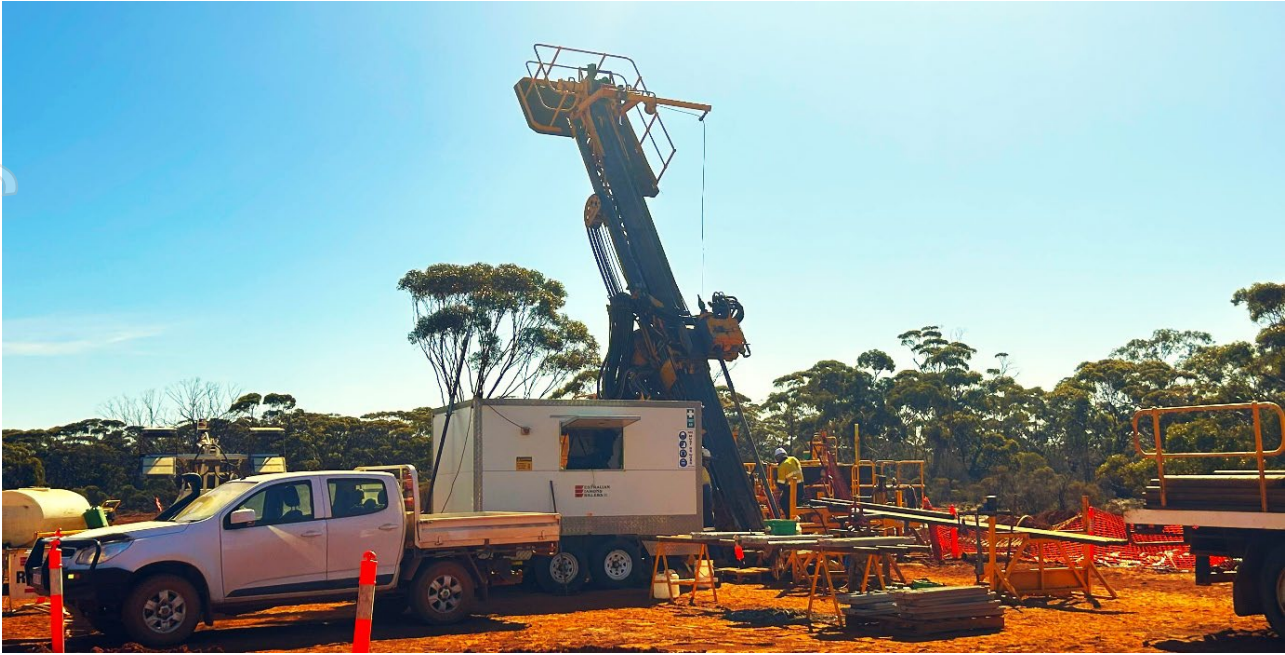
Image 2 – Diamond drill rig at Kamperman (November 2023).
