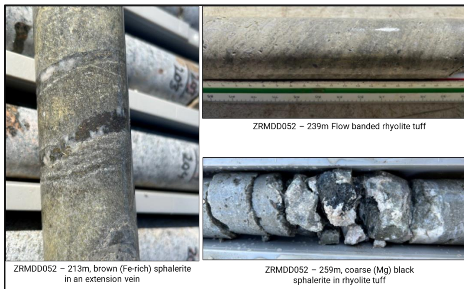
Figure 6: Examples of key lithologies and veins encountered in ZMRDD052 (118m @0.54 g/t Au from 225m)
